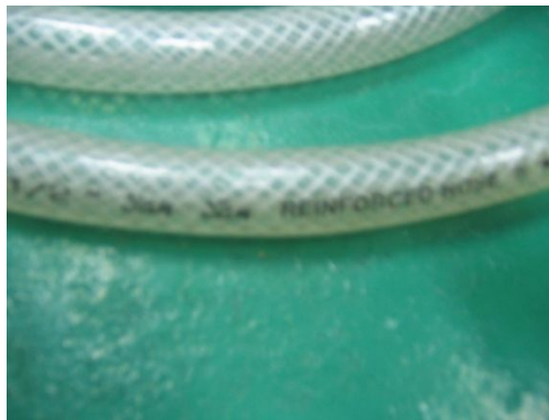
FIGURE 3.4: Pipe Hose to Supply Air
