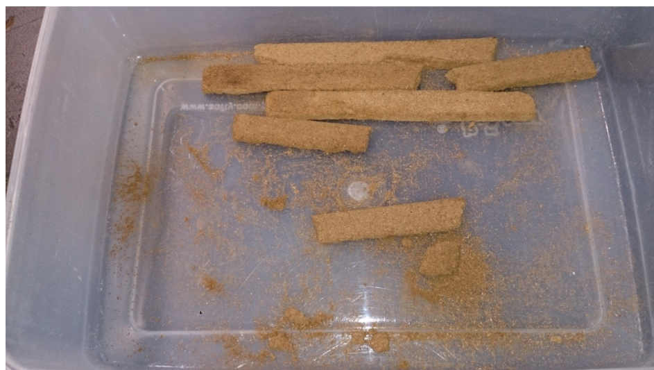
FIGURE 20: Biocomposite films made from raw OPF under temperature 210°C, pressure 20Mpa, compression time 10min.
