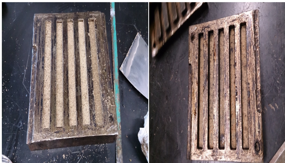
FIGURE 25: (Left) Biomass before thermal compression. (Right) Biocomposite boards produced after thermal compression. (Mold column from left to right: EmimDEP, BmimCl, EmimAc, Water, BmimTFMS).
