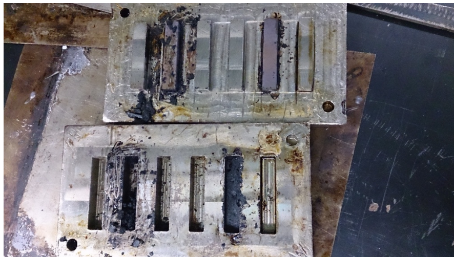
FIGURE 16: Result of first trial- OPEFB/IL turned into black charcoal at temperature 200°C, pressure 20MPa, time 20min.
