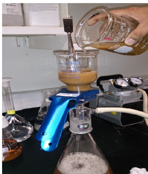
FIGURE 18: Regenerating OPF using vacuum filtration.
