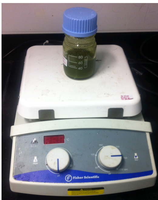
FIGURE 7: Mixing with Magnetic Stirrer
