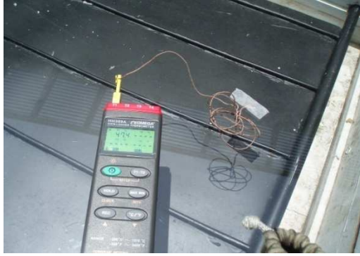
Figure 3.11 Thermocouple and data logger used for the experiment
