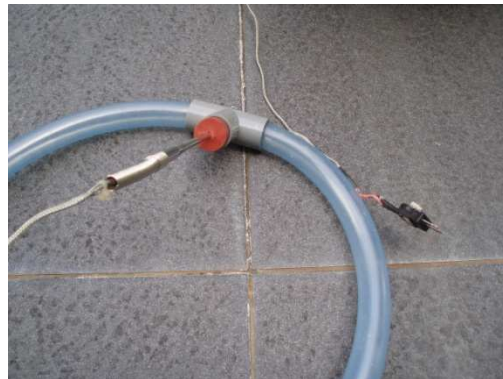
Figure 3.13 Connector with thermocouple to measure water temperature
