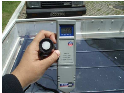
Figure 3.10 Pyranometer used to measure the solar radiation
