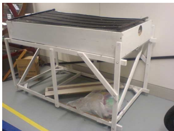
Figure 3.5 Flat Plate Solar Collector available in the lab
