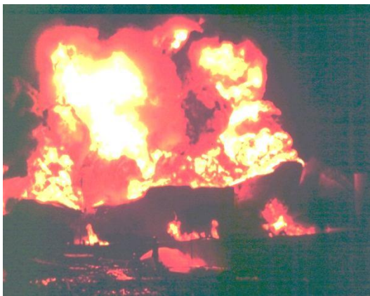
Figure 1.1: Slopover tank fire. [2]
