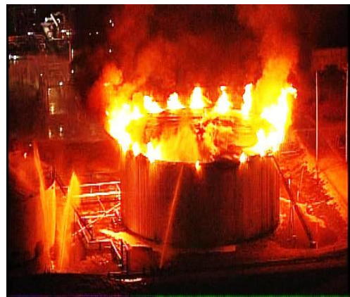
Figure 1.2: Frothover tank fire [2]
