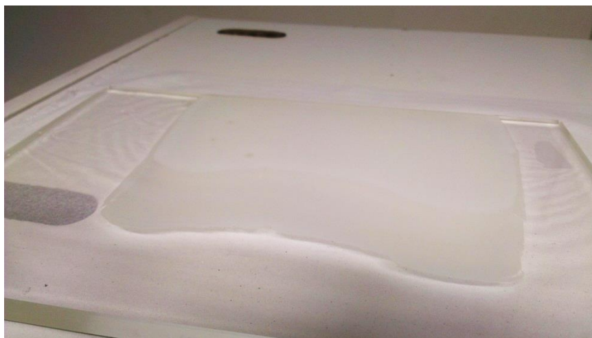
Figure 10: Wet phase inversion membrane fabrication experiment set up
