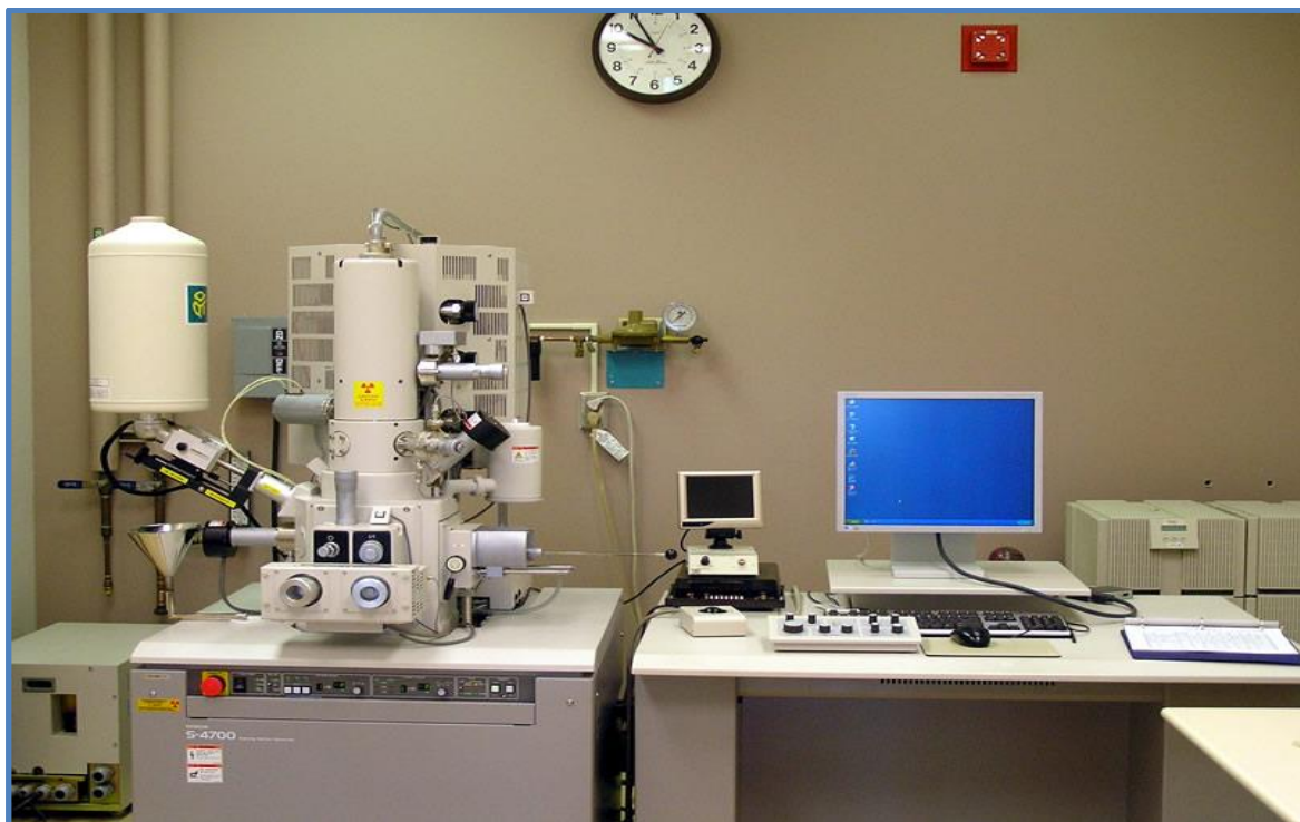
Figure 9 : Field Emission Scanning Electron Microscopy machine
