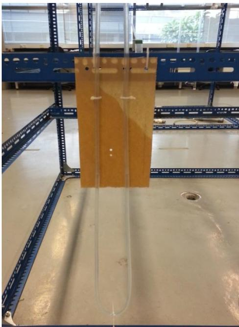
**Figure 11:** Orifice flow metre pressure difference manometer
