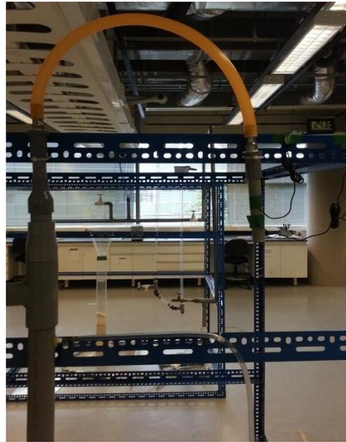
**Figure 10:** Gas outlet with digital thermometers
