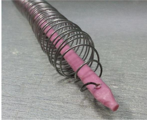
**Figure 6:** Connection of wire onto the rod of Helix Prime
