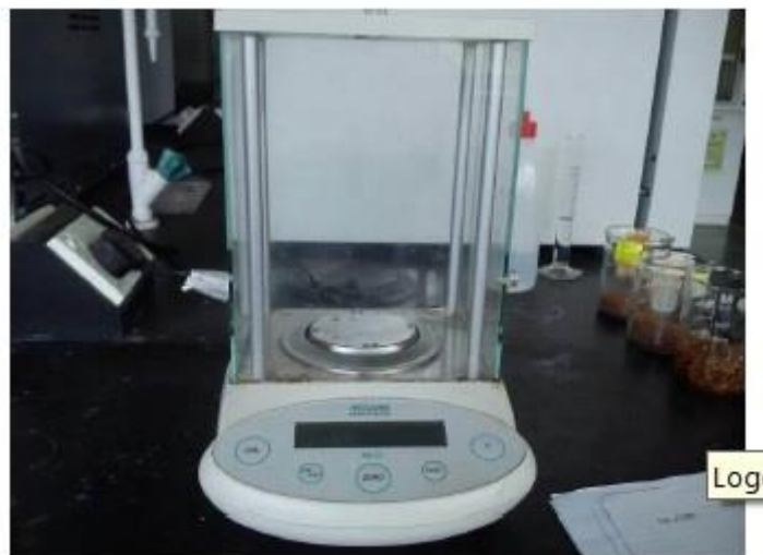
Figure 11: Weighing balance to weight the sawdust particle
