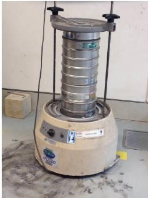
Figure 10: Sieving machine to sieve the sawdust
