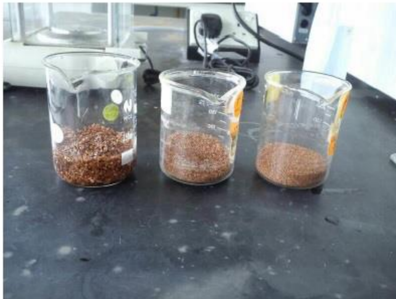
Figure 13: Dried sawdust after being in oven for 24 hours
