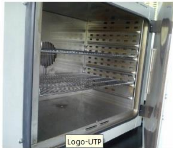
Figure 12: Oven used to dry sawdust at 100 °C
