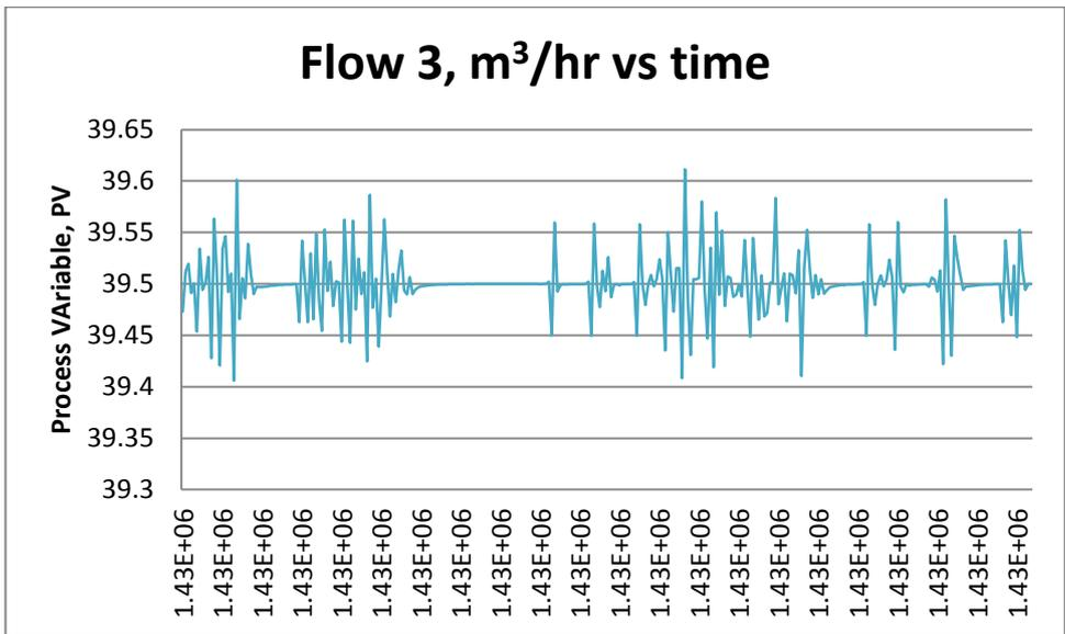
Figure 4.12: Response of Flow 3 controller during step test.
