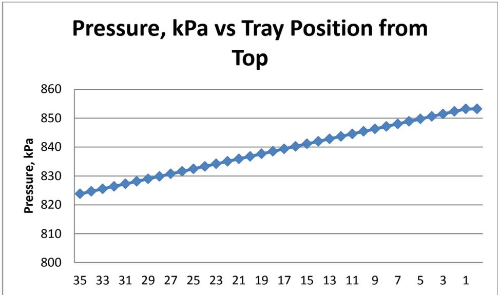
Figure 4.4: Debutanizer Pressure versus Tray position from Top at Steady state.
