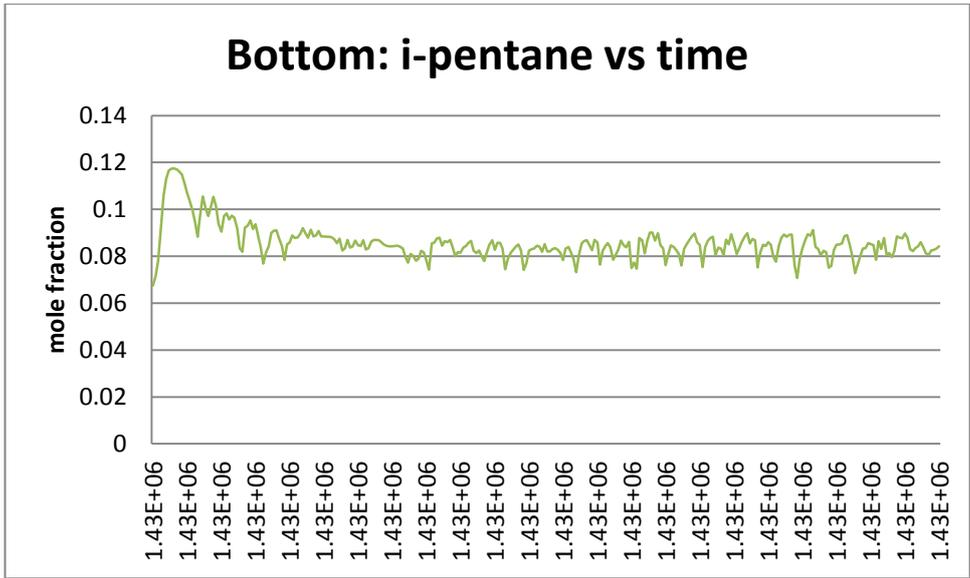
Figure 4.19: Mole fraction of i-pentane at the bottom exit of Debutanizer.
