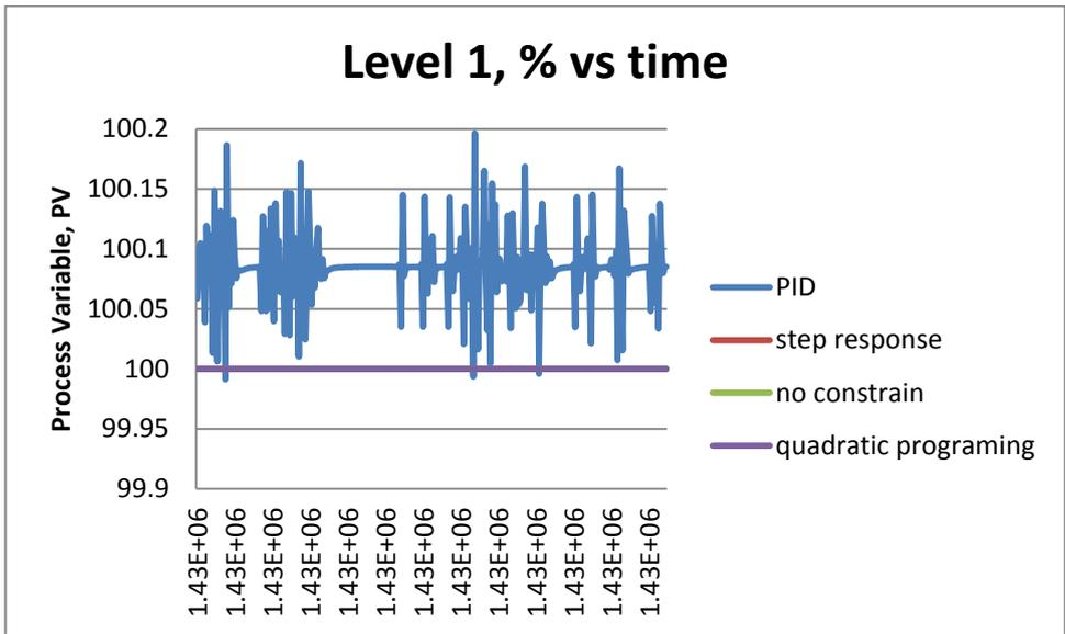
Figure 4.44: Comparison of Level 1 controllers' response.
