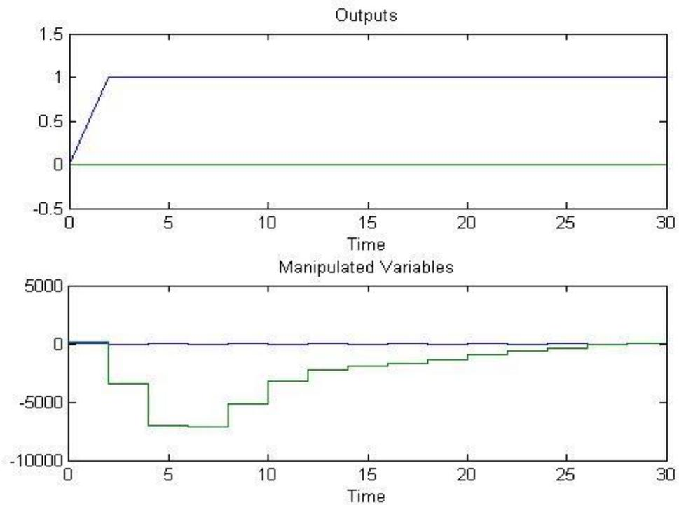
Figure 4.26: Feed Flow Controller response
