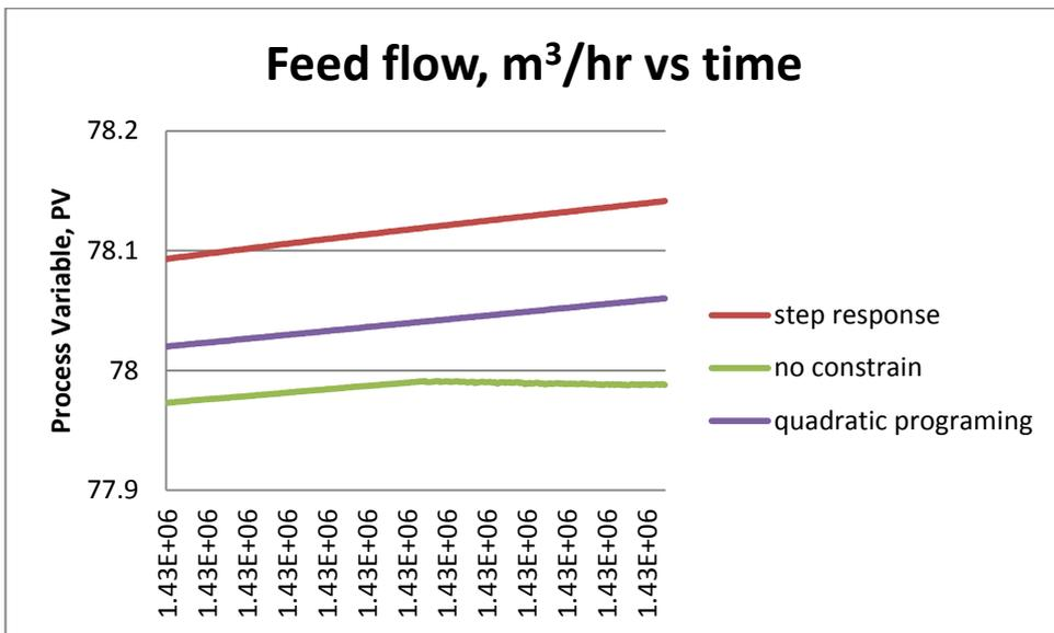
Figure 4.40: Comparison of Feed Flow - MPC controllers' response.
