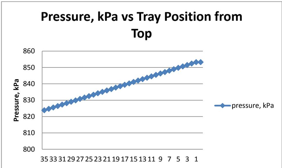
Figure 4.5: Debutanizer Pressure versus Tray Position from Top at Dynamic state.
