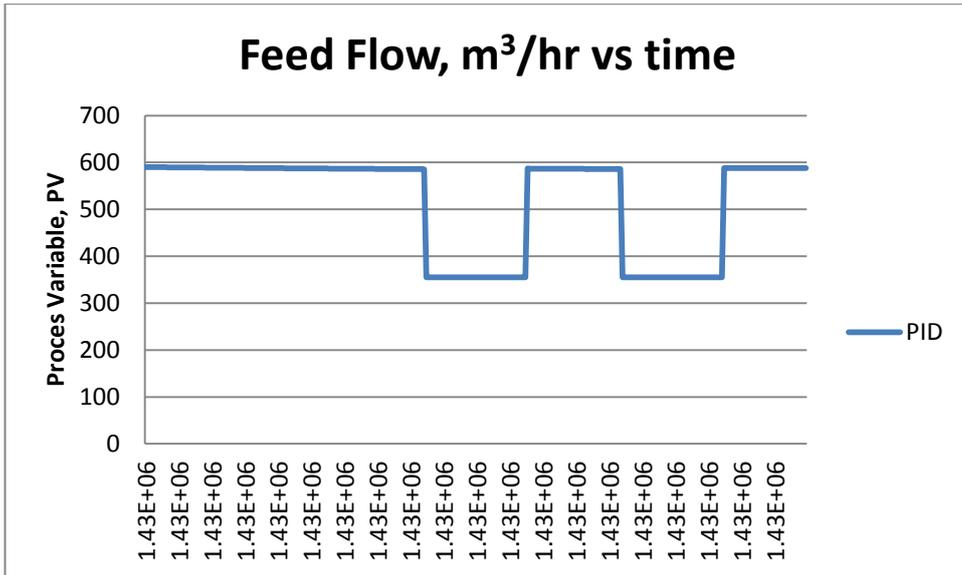
Figure 4.39: Feed Flow - PID controller response.
