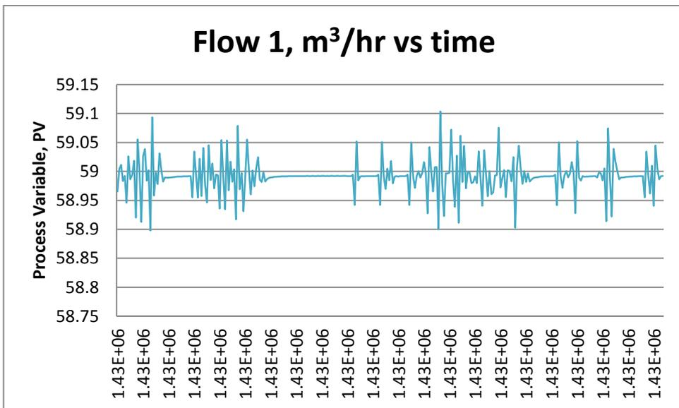
Figure 4.10: Response of Flow 1 controller during step test.
