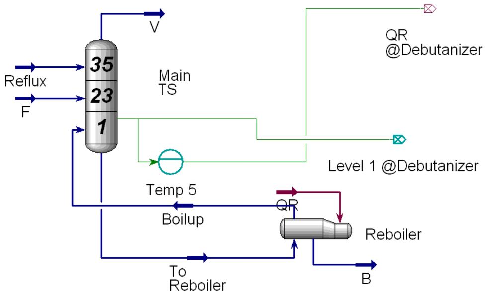
Figure 4.2: Distillation Column built in HYSYS™ software
