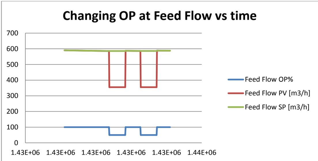
Figure 4.9: Details of Feed Flow controller during step test.
