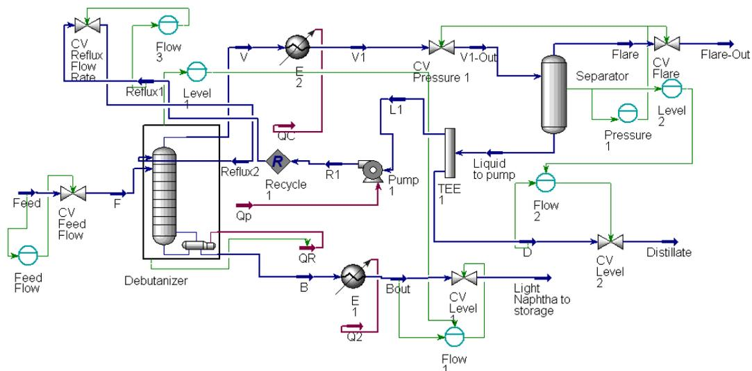
Figure 4.3: Dynamic model built in HYSYS™ software
