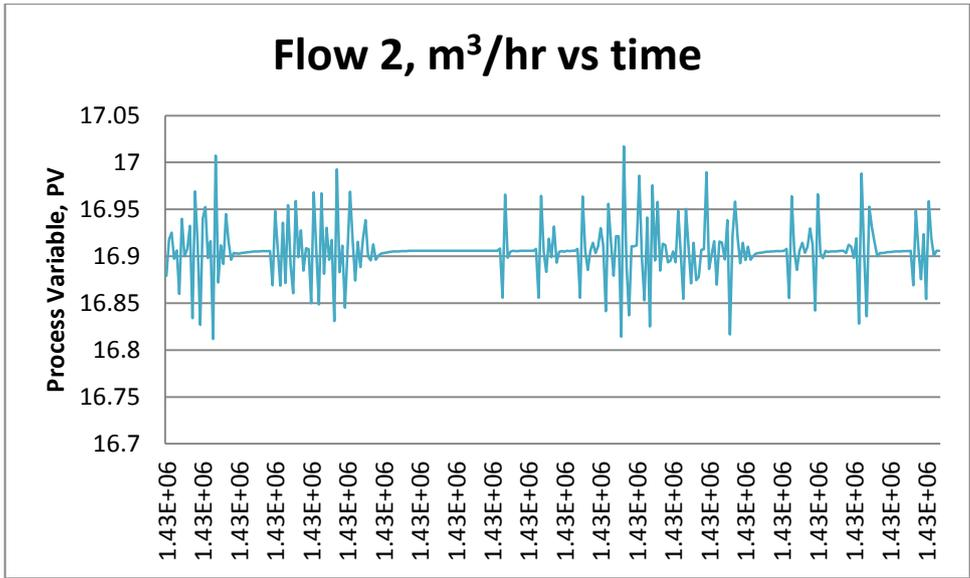
Figure 4.11: Response of Flow 2 controller during step test.
