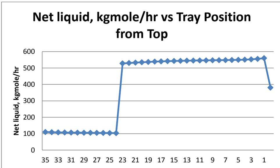
Figure 4.7: Debutanizer Net liquid, kgmole/hr versus Tray Position from Top at Dynamic state.
