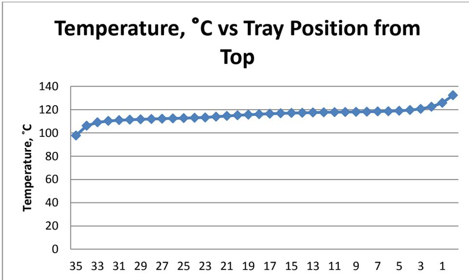
Figure 4.6: Debutanizer Temperature, °C versus Tray Position from Top at Dynamic state.
