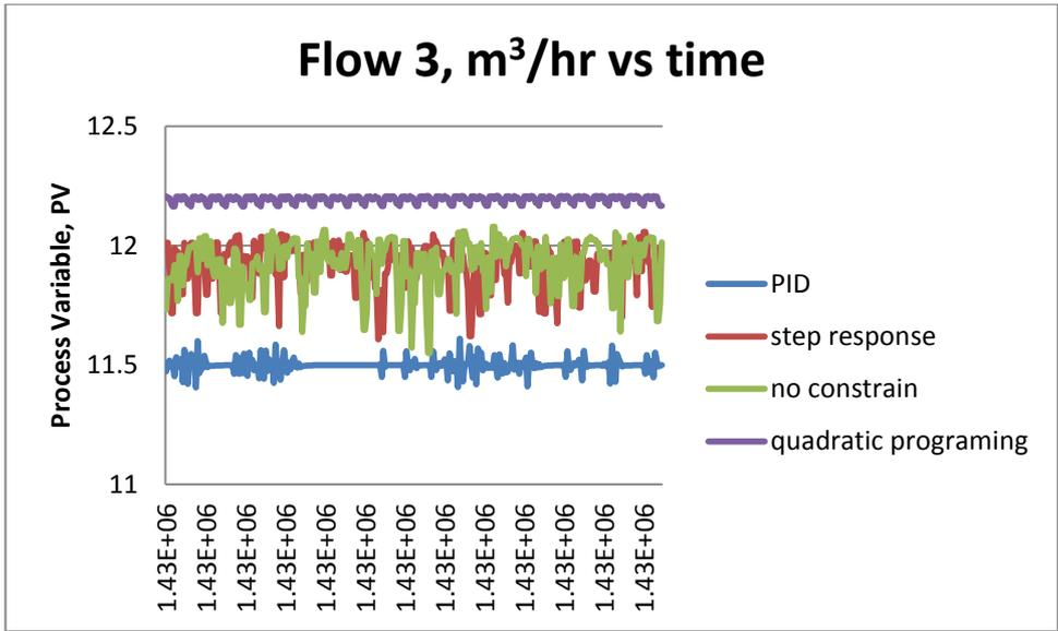
Figure 4.43: Comparison of Flow 3 controllers' response.
