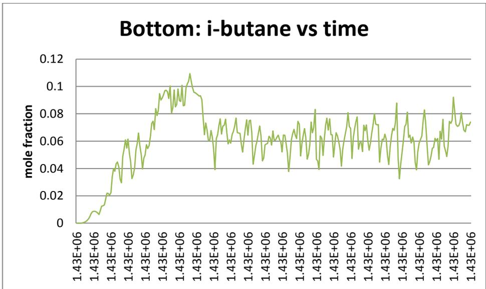
Figure 4.20: Mole fraction of i-butane at the bottom exit of Debutanizer.
