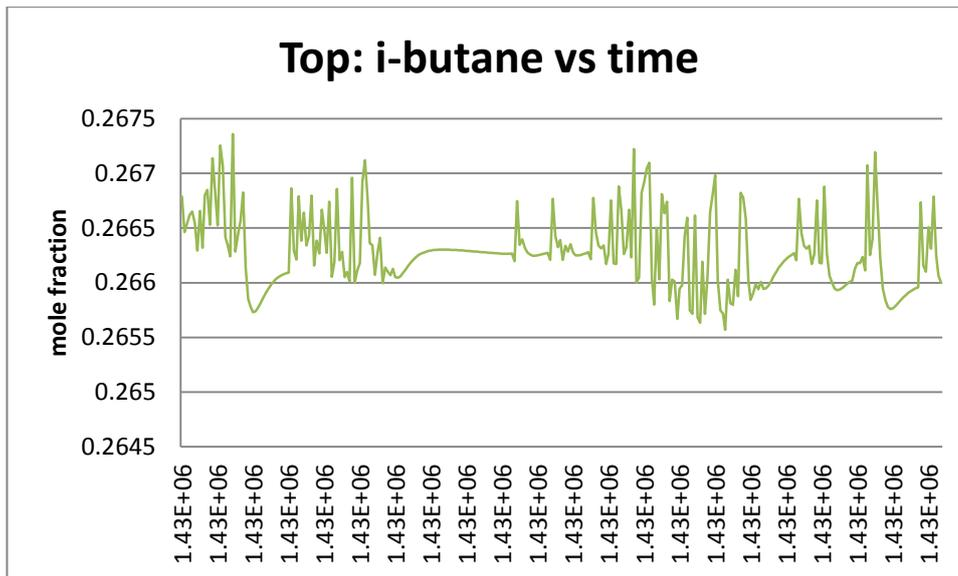
Figure 4.25: Mole fraction of i-butane at the top exit of Debutanizer.
