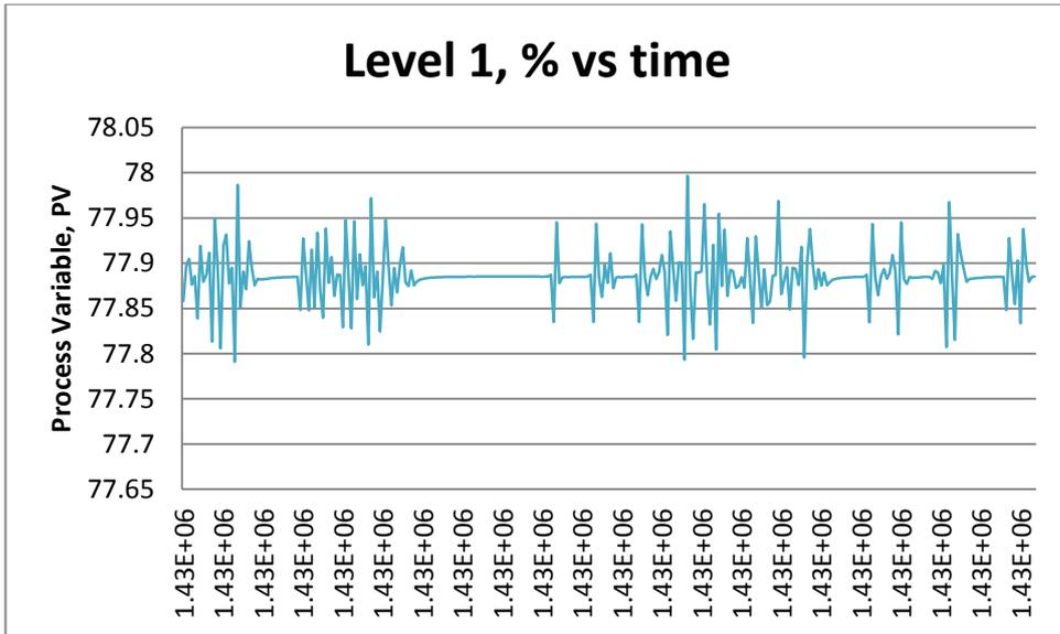
Figure 4.13: Response of Level 1 controller during step test.
