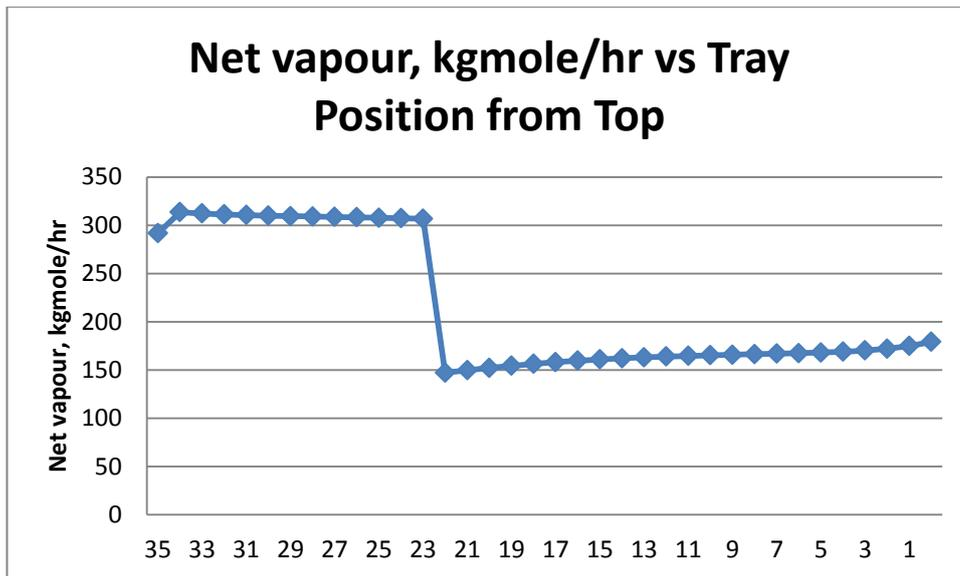
Figure 4.8: Debutanizer Net vapour, kgmole/hr versus Tray Position from Top at Dynamic state.
