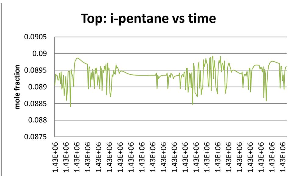
Figure 4.24: Mole fraction of i-pentane at the top exit of Debutanizer.
