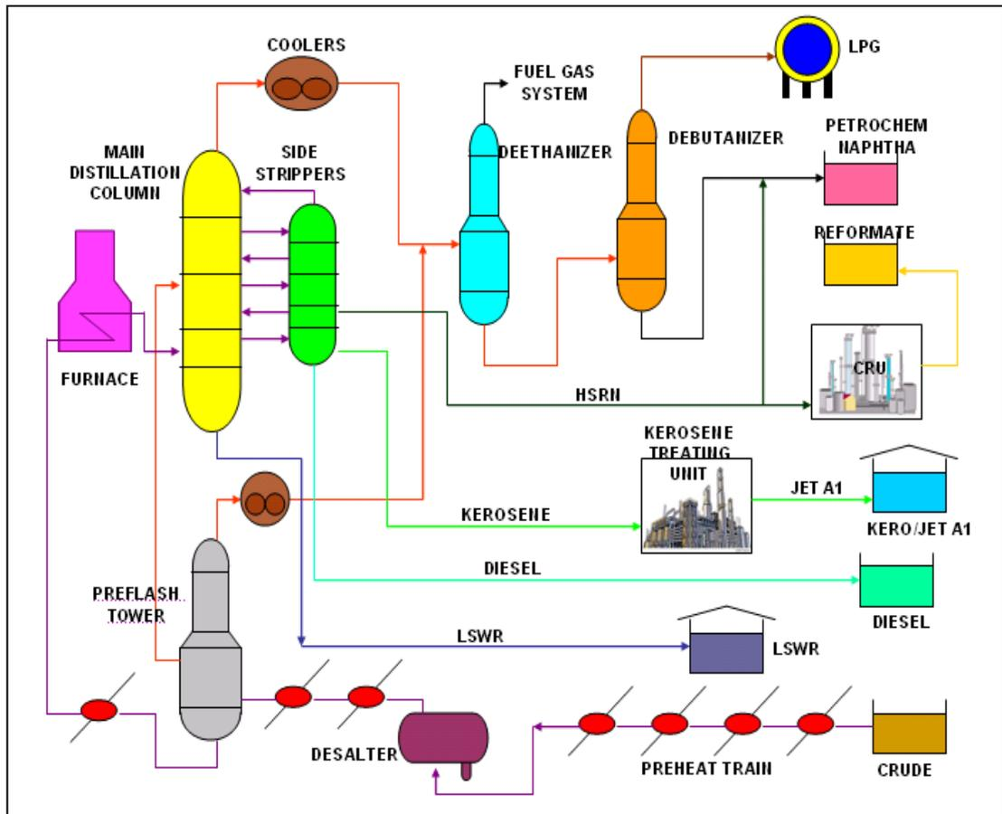
Figure 1.2: Process Flow Diagram (PFD) of Crude Distillation Unit (CDU)
