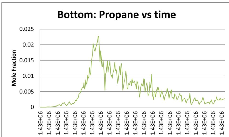
Figure 4.16: Mole fraction of propane at the bottom exit of Debutanizer.
