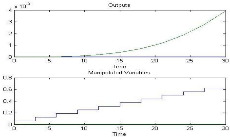
Figure 4.36: Level 1 Controller response
