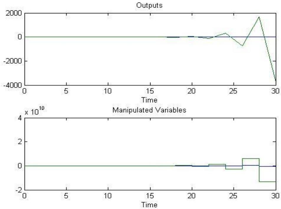
Figure 4.27: Flow 1 Controller response
