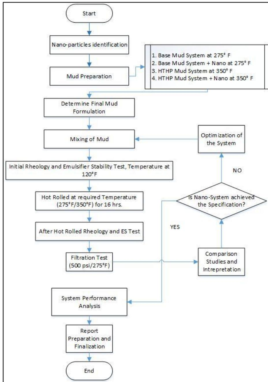
**Figure 3: Process flowchart for nano SBM**
