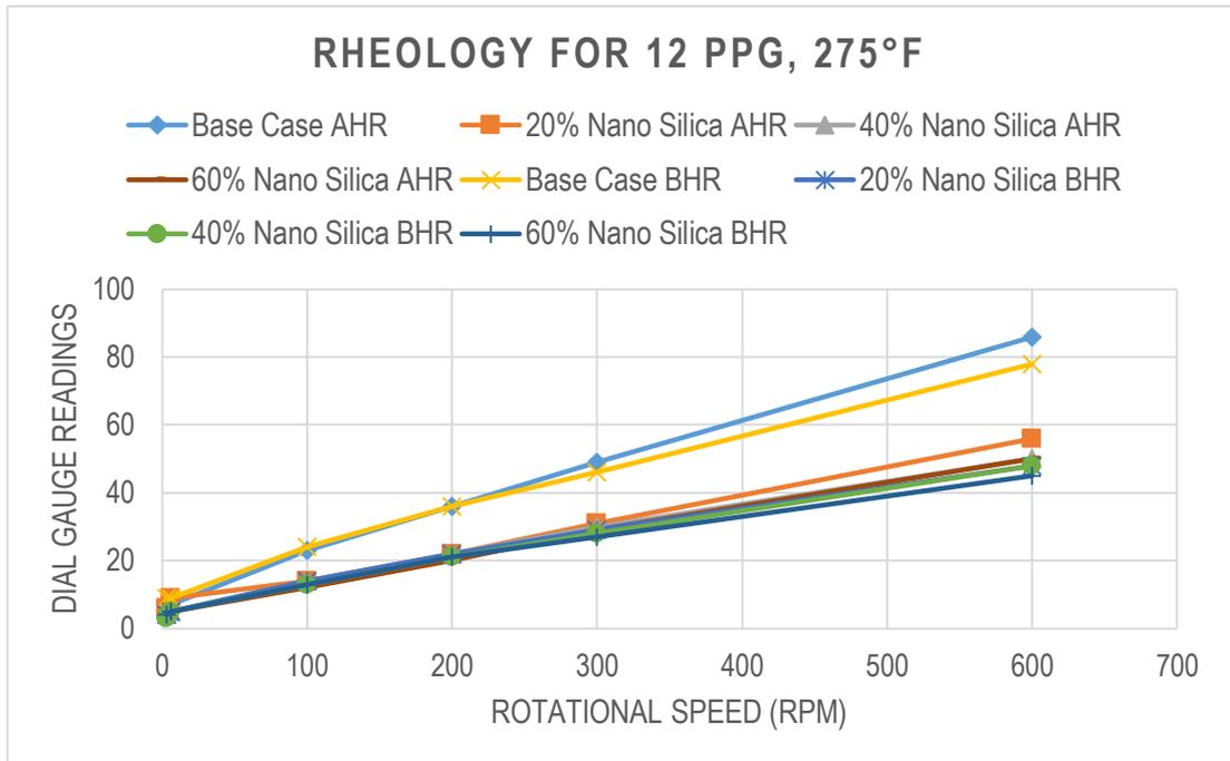
**Figure 6: Dial readings vs. RPM for 12 ppg, 275°F mud system**
