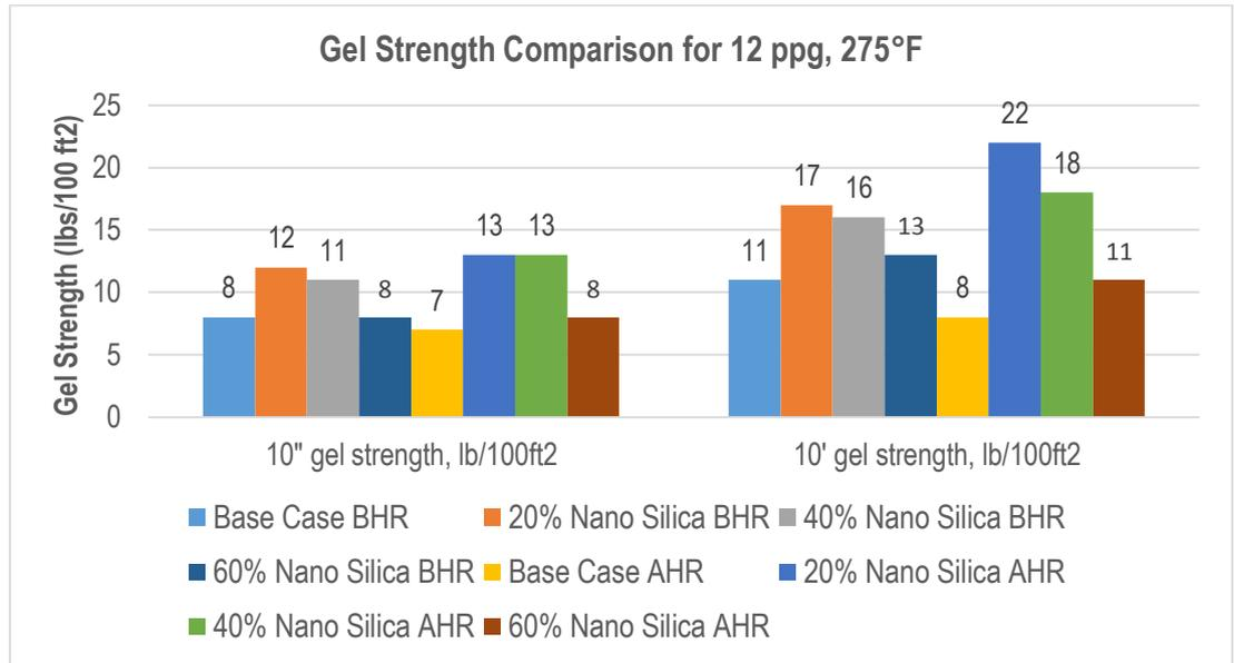
**Figure 10: Gel strength comparison for 12 ppg, 275°F mud**
