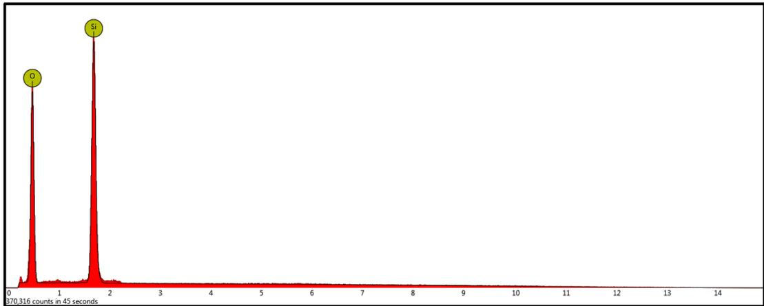
**Figure 5: EDS analysis for nano silica elemental identification**
