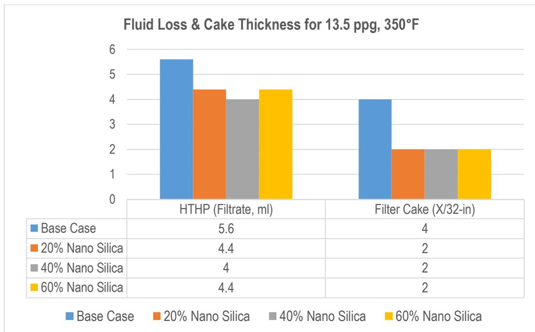
**Figure 13: Fluid loss and mud cake thickness for 13.5 ppg, 350°F mud**
