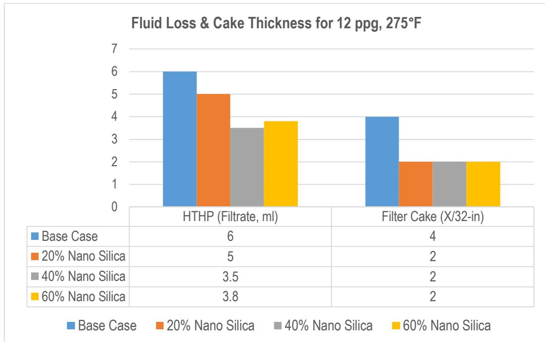
**Figure 12: Fluid loss and mud cake thickness for 12 ppg, 275°F mud**
