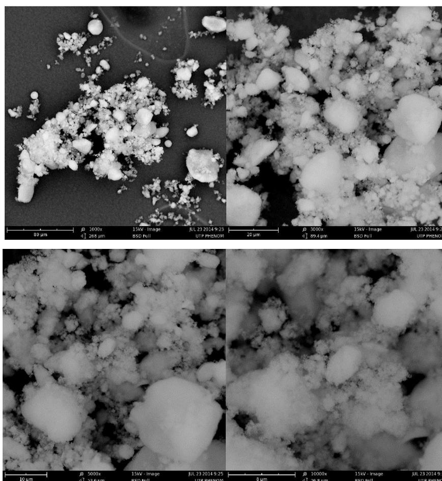
**Figure 4: SEM images of nano silica, from top left: Magnification of 1000x, 3000x, 5000x, 10000x**
