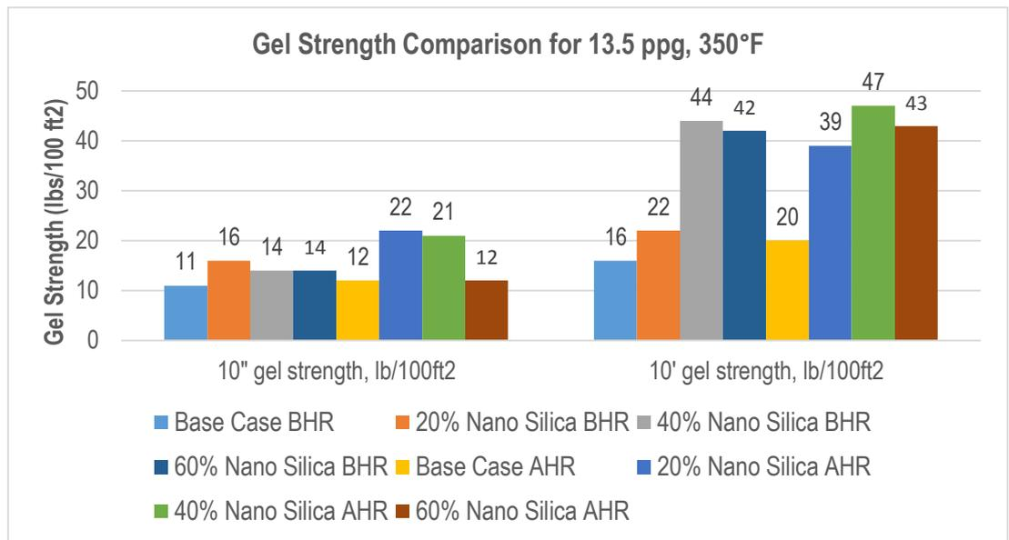
**Figure 11: Gel strength comparison for 13.5 ppg, 350°F mud**
