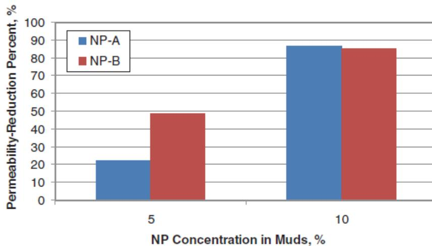
**Figure 2: Effect of nano particles concentration in muds on permeability-reduction percent [30]**
