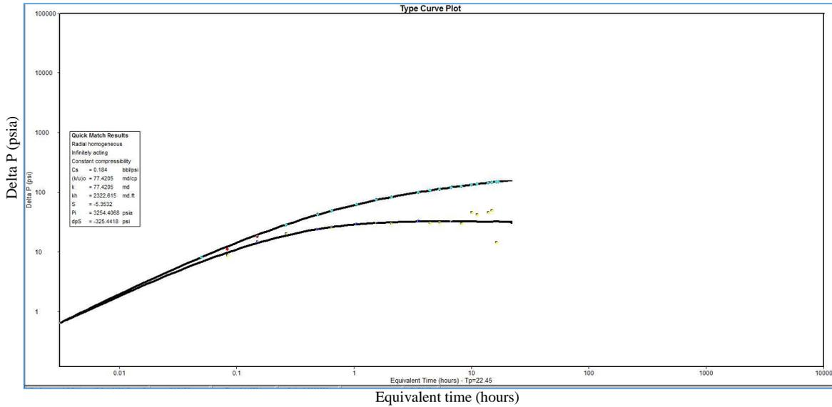
FIGURE 11. Auto-Matching From Type Curve Analysis
