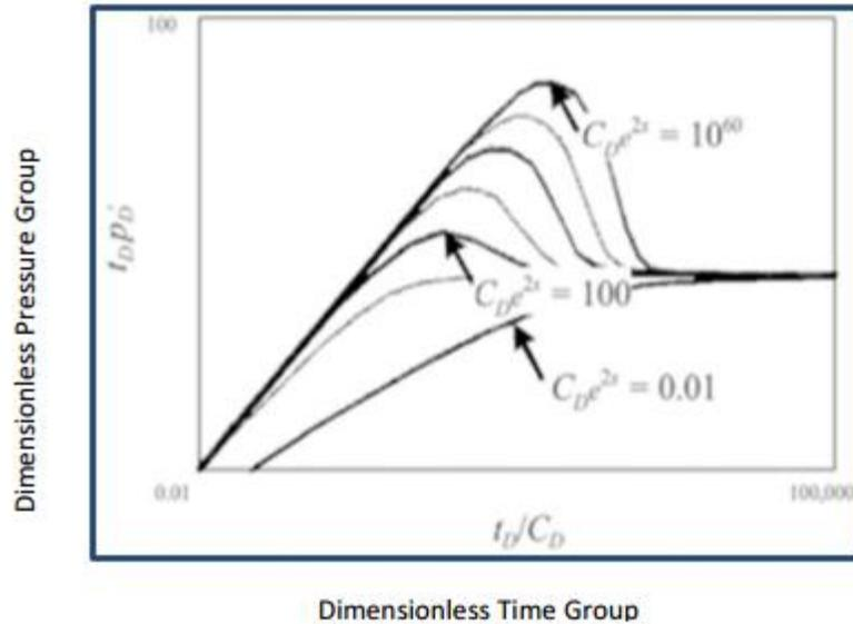
FIGURE 3. Derivative Type-Curve for Infinite Acting Reservoir
