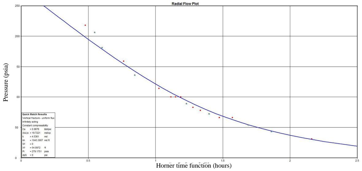
FIGURE 15. Auto Match on Radial Flow Rate Plot (Hydraulically Fractured Well)
