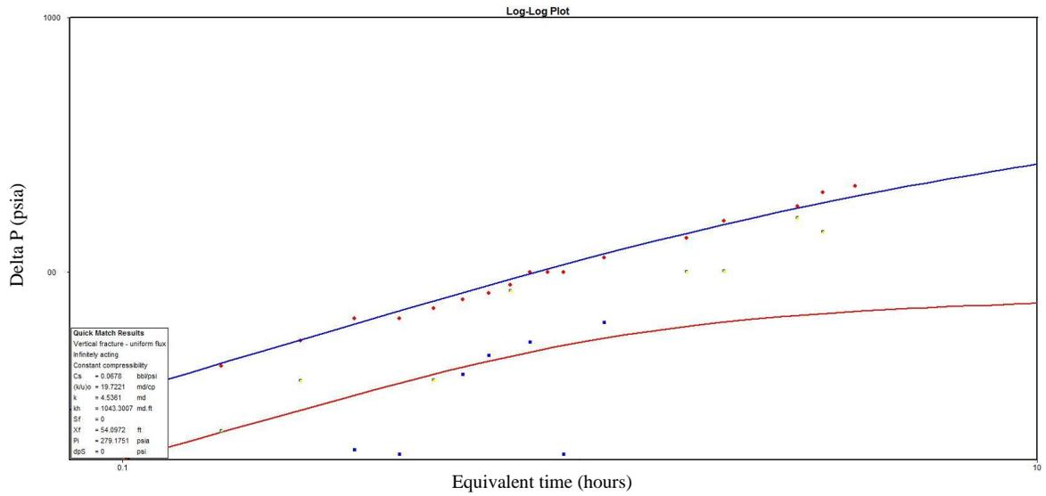
FIGURE 13. Log-log Plot of Delta Pressure Versus Equivalent Time (Hydraulically Fractured Well)
