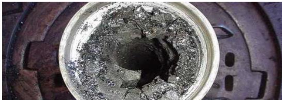
Figure 2 : Asphaltene precipitation deposited inside pipe
