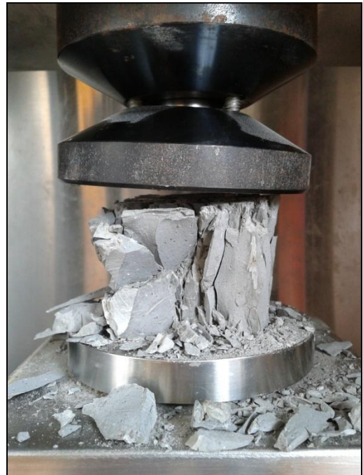
Compressive Strength Tester (left); Crushing of Cement Sample (right)
