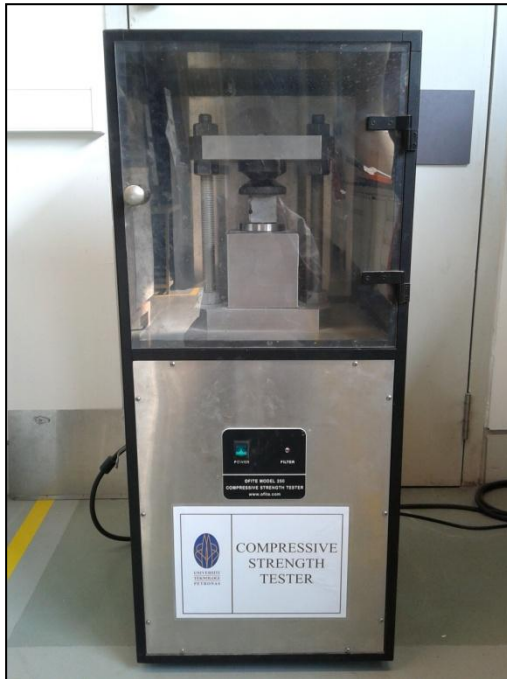
Compressive Strength Tester (left); Crushing of Cement Sample (right)
