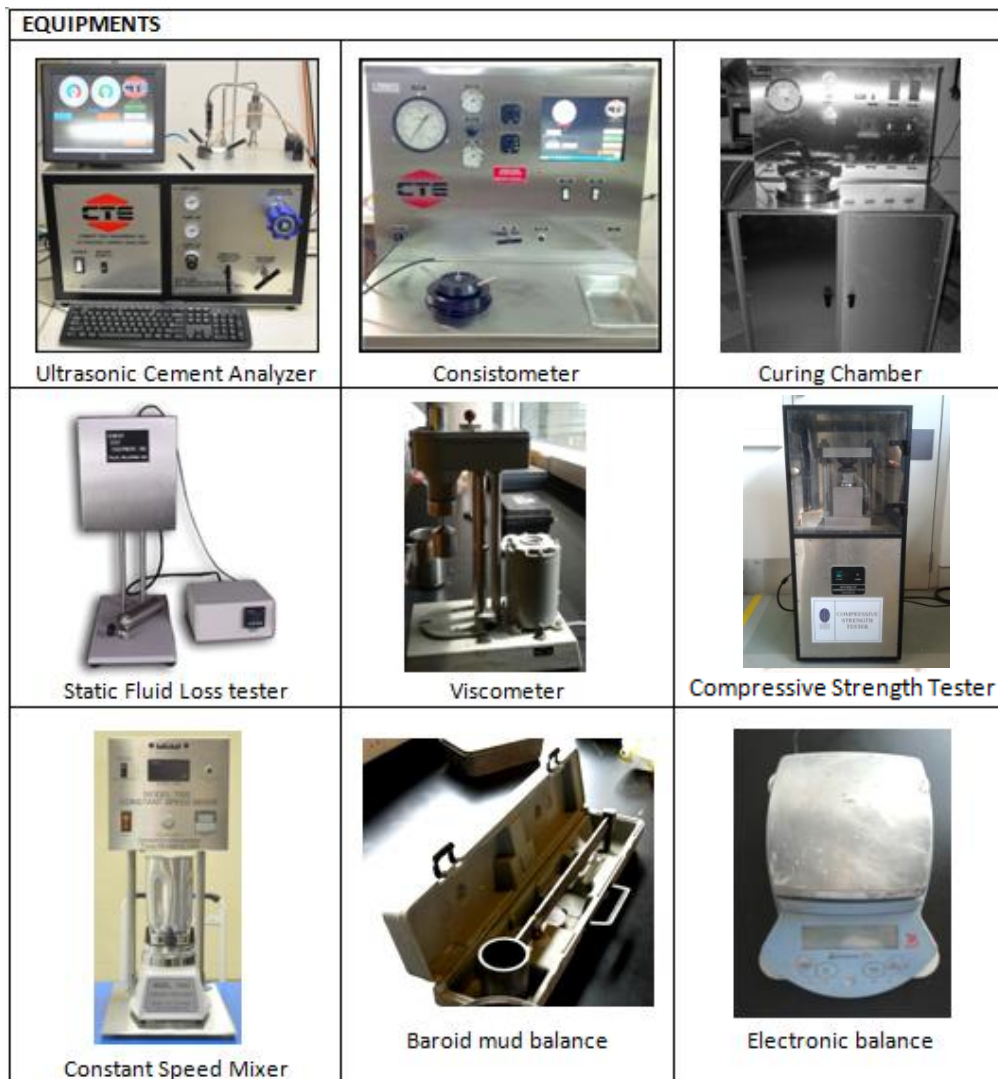
FIGURE 3.2: Equipments for slurry preparation
