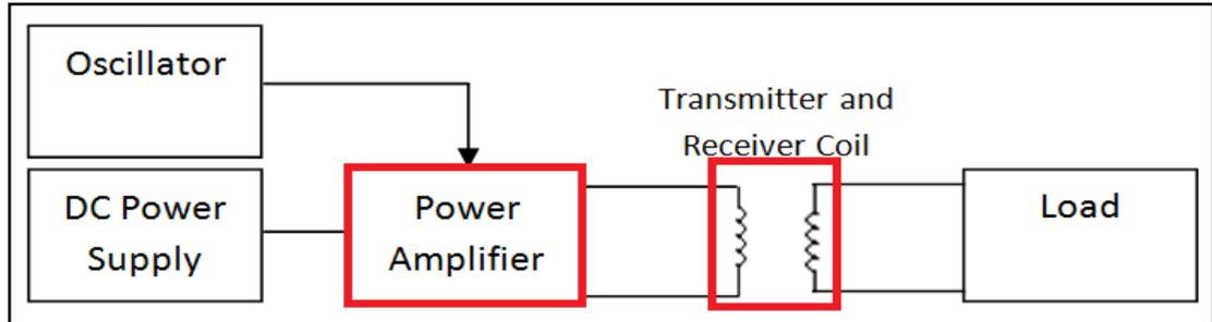
Figure 1 : Wireless Power Transmission System Summary
