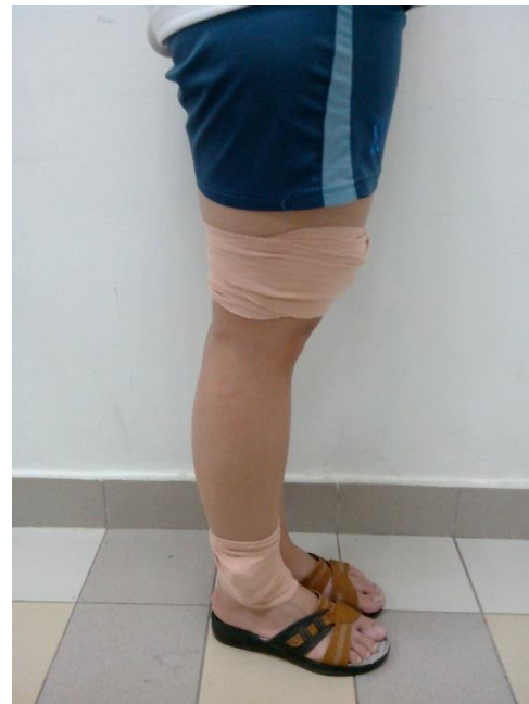
Figure 16: Subject under test with two-sensor-node-system (thigh and ankle) for standing activity where sensors are secured in position with reusable bandage
