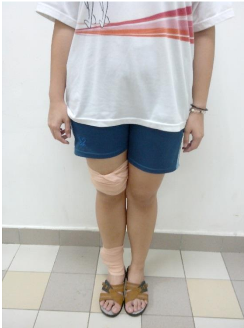
Figure 16: Subject under test with two-sensor-node-system (thigh and ankle) for standing activity where sensors are secured in position with reusable bandage
