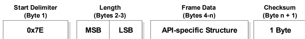
Figure 3-01. UART Data Frame Structure:
