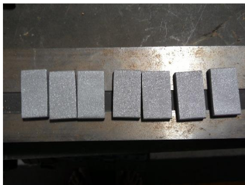
Figure 4: Substrate metal after sandblasting Figure 5: Substrate metal after HVOF
