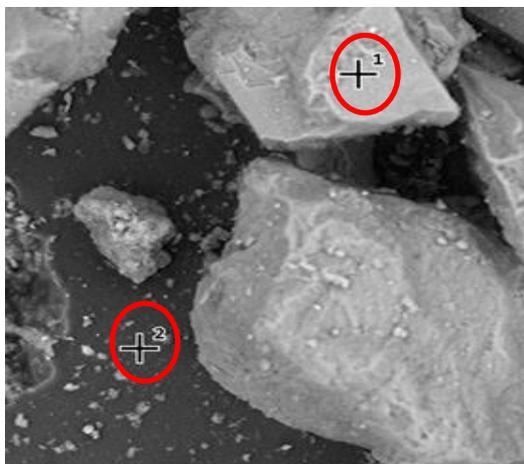
Figure 4.13. Spectrum 1 and 2 shows the surface points of the siliconized sample where the EDX is performed.
