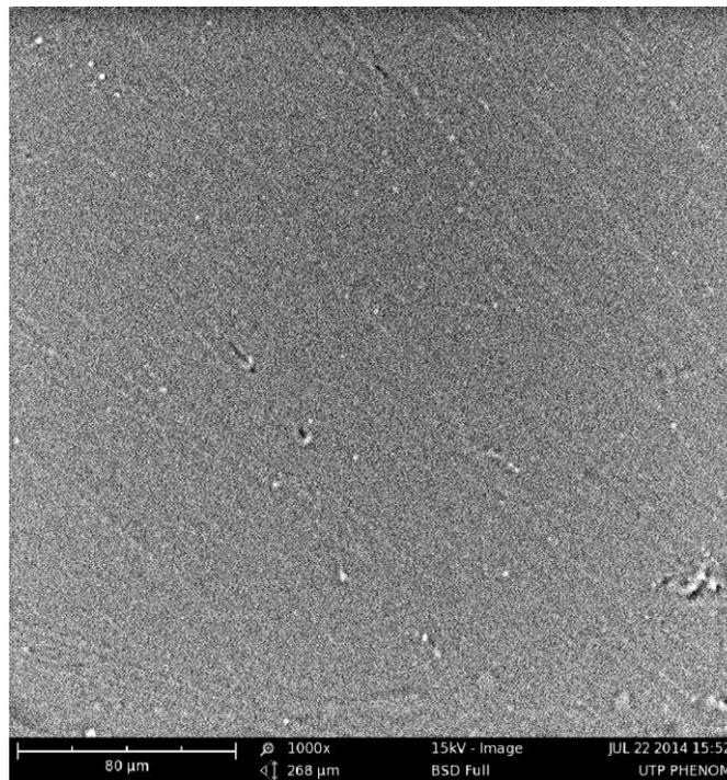
Figure 4.6. Morphology of acrylic surface before siliconizing process.
