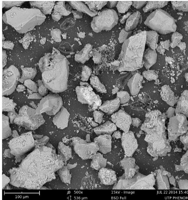
Figure 4.7. Morphology of acrylic surface after siliconizing process at 160°C.
