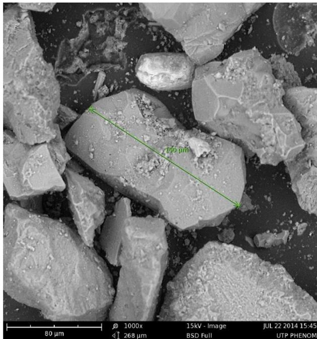
Figure 4.9. Size of silica sand
