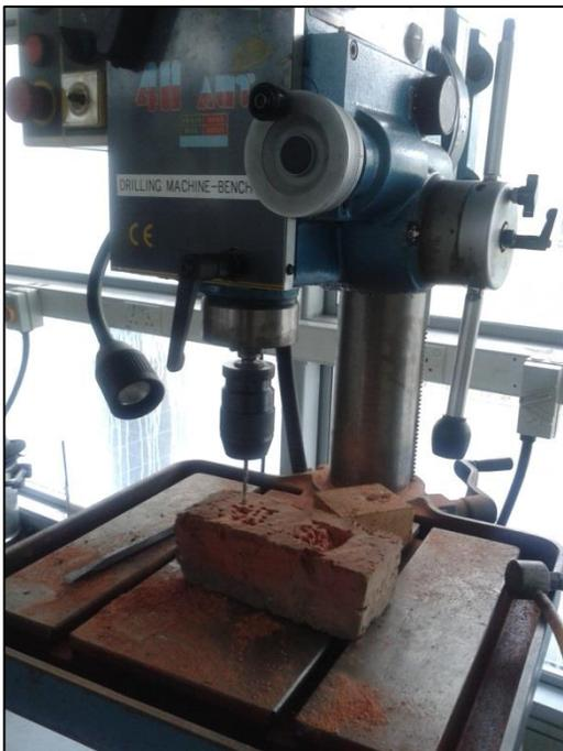
Figure 3.5. Milling process of the pockets
