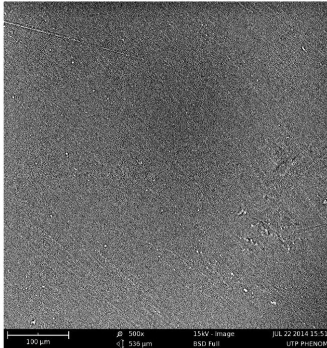
Figure 4.5. Morphology of acrylic surface before siliconizing process.
