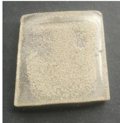
Figure 4.3. Sample after siliconizing
