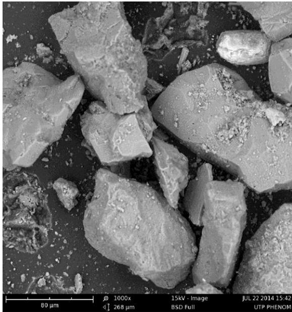
Figure 4.8. Morphology of acrylic surface after siliconizing process at 160°C.
