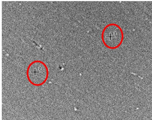
Figure 4.10. Spectrum 1 and 2 shows the surface points of the sample where the EDX is performed.
