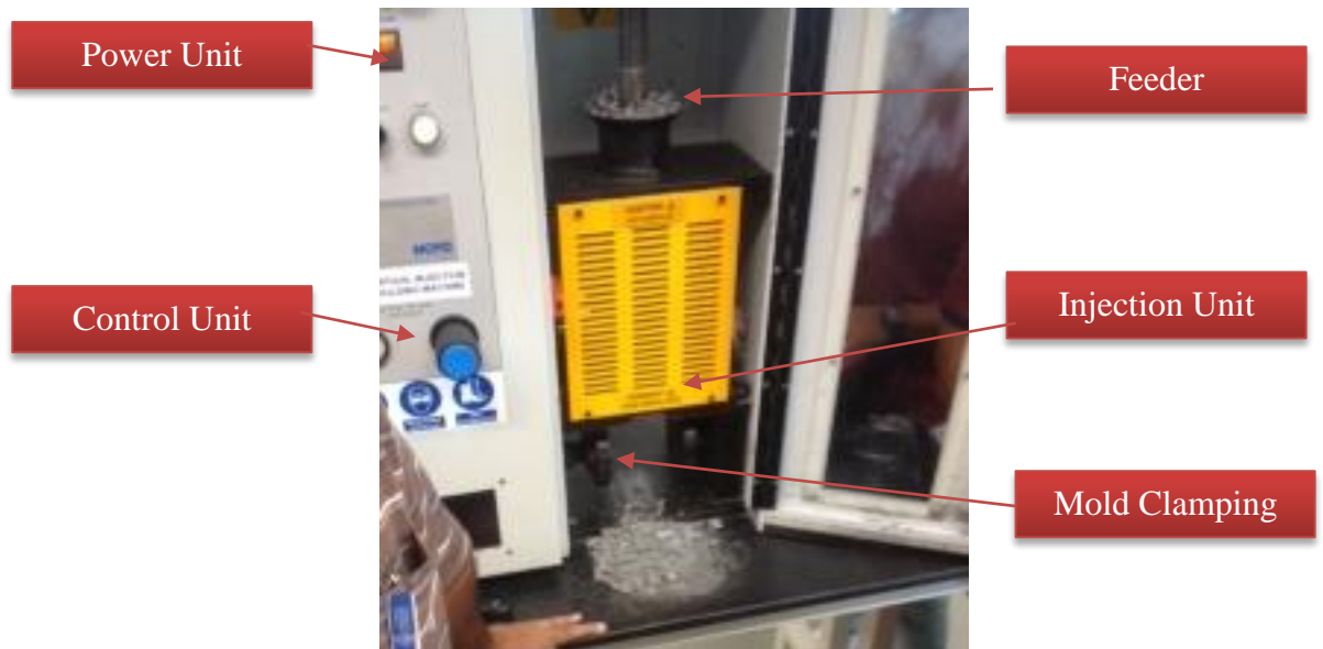
Figure 3-4: Components of injection molding
