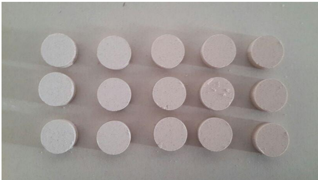
Figure 3.11: Compressed samples before heating inside an oven
