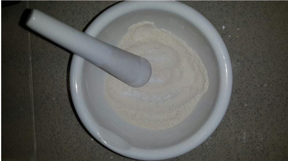
Figure 3.10: Mixture of sand dust and calcium carbonate in a ceramic mortar
