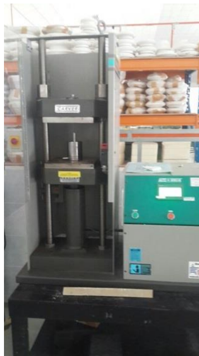
Figure 3.5: Compressor used to compress the samples
