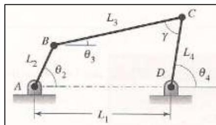
Figure 2.7: Basic four-bar linkage mechanism
