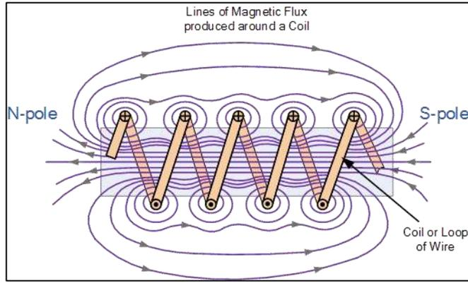
Figure 2.5: Electromagnet Line Force
