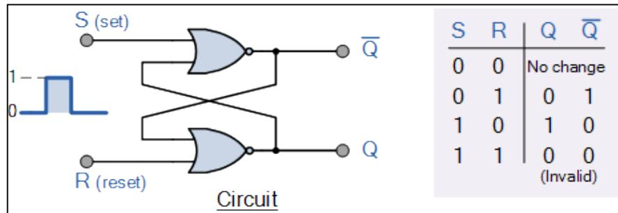
Figure 2.9: NOR Gate SR Flip-Flop Truth Table
