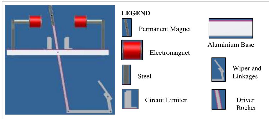
Figure 1.1: Schematic diagram of windshield wiper
