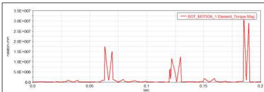
Figure 4.8: Torque magnitude at 1:0.9 ratio
