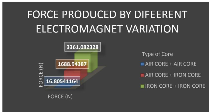
Figure 4.2: Force Generated by Different Electromagnetic Setup
