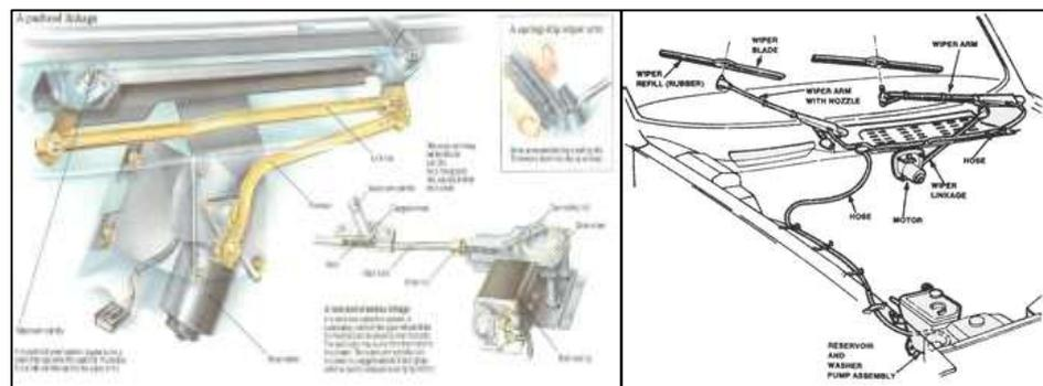
Figure 2.4: Car Wipers Linkage Mechanism
