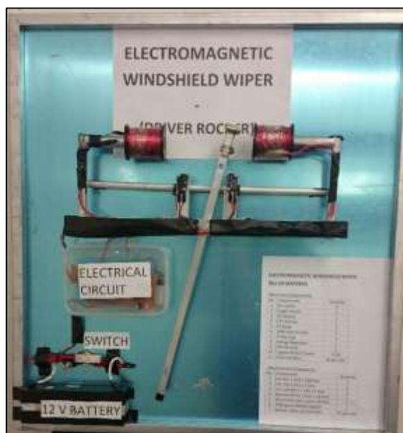
Figure 3.18: Driver rocker Assembly
