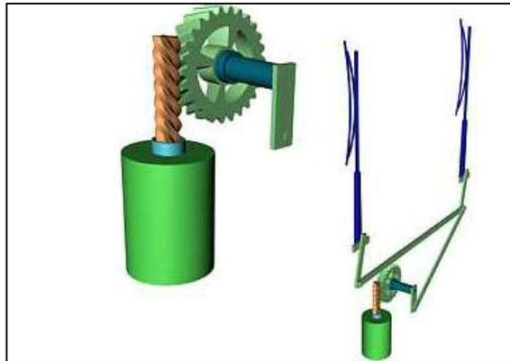
Figure 2.3: Car Wipers Working Mechanism
