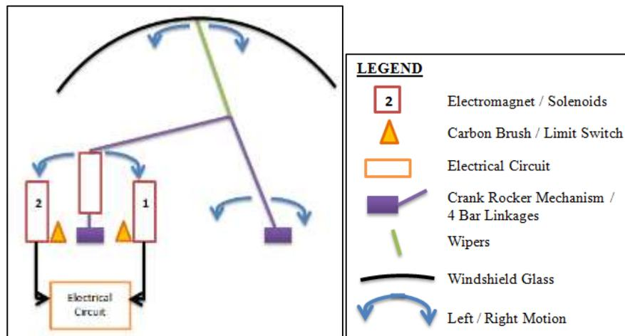
Figure 3.3: Basic Wiper Concept
