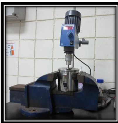
Figure 3: Preparation of emulsified fuel
