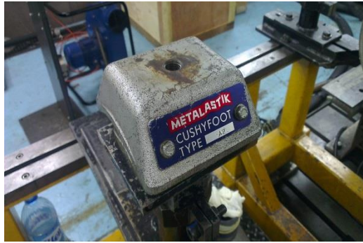
Figure 5.1: Example of combined spring and flexible mount
