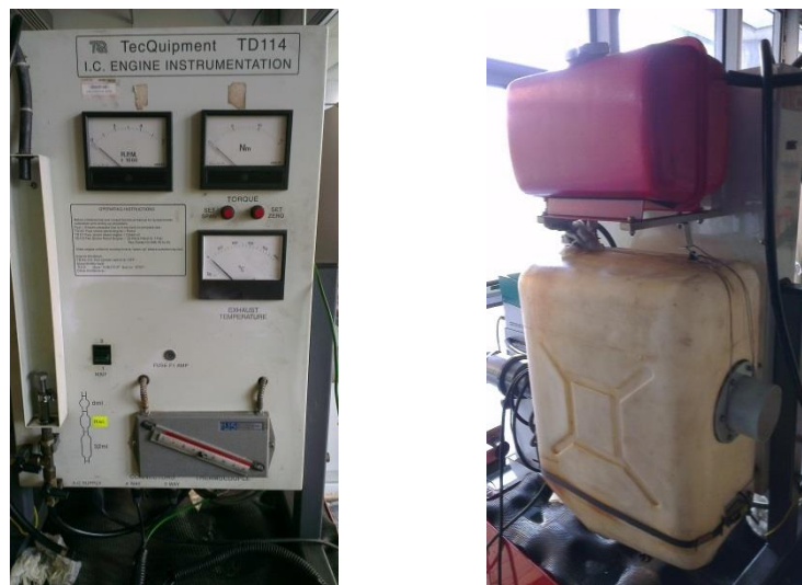
Figure 3.2: Test bed instrumentation unit. Consisted of speed meter, torque meter, exhaust temperature meter, air flow meter, fuel tank, and water tank
