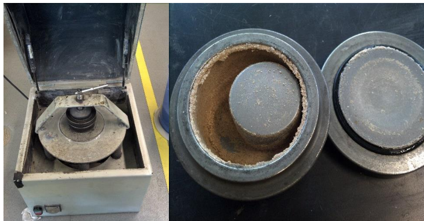
Figure 5: Cole Parmer Mortar Grinder. [15]
