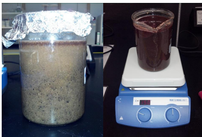
Figure 7: CR powder cooked with 1M NaOH at 150°C mixture temperature.
