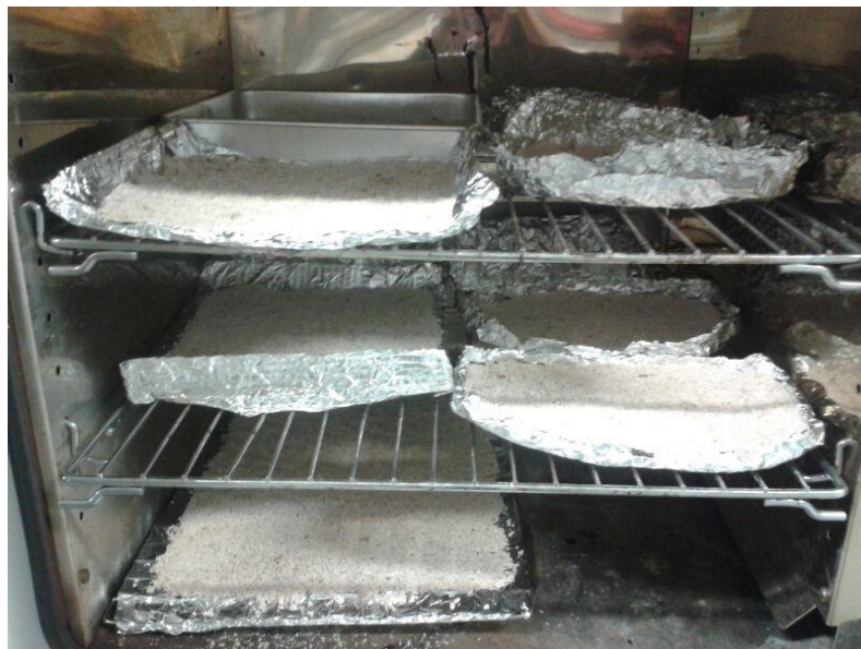
Figure 3: Washed CR was oven-dried for 30 minutes.
