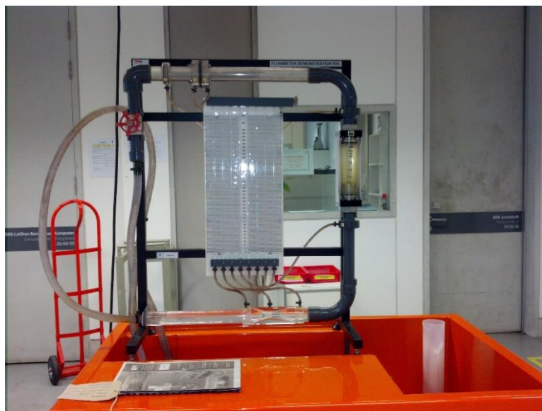
Figure 13: Flowmeter experimental setup with Orifice plate.
