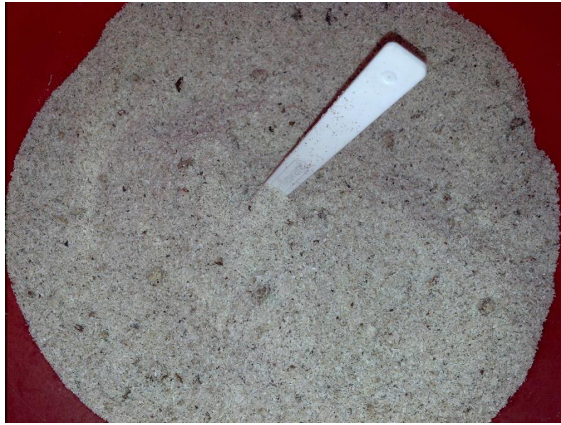
Figure 4: CR after dried in the oven for 30 minutes at 121°C (250°F).
