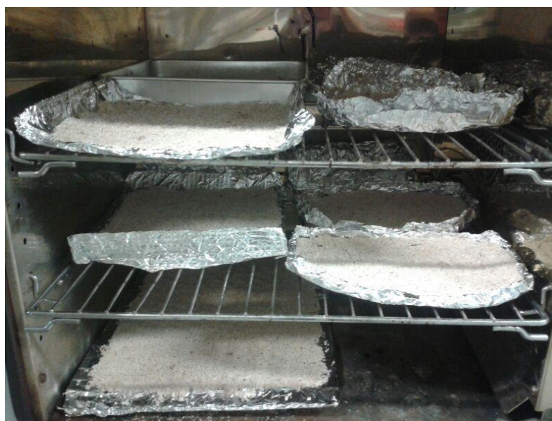
Figure 10: Residues were oven-dried for 30 minutes at 121°C (250°F).
