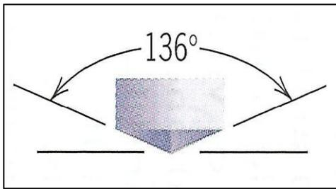
Figure 2.7: Shape of Indentation (side view)
