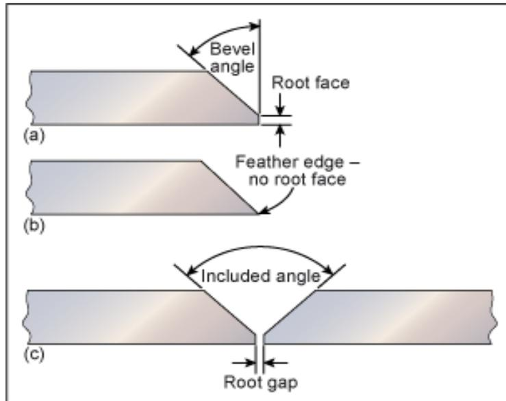
Figure 3.2: Bevel preparation illustration
