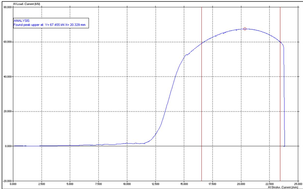
Figure 4.14: Force versus Strain for SA106B Steel (Before Heat Treatment)
