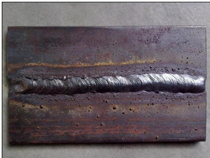
Figure 3.5: Shielded Metal Arc Welding
