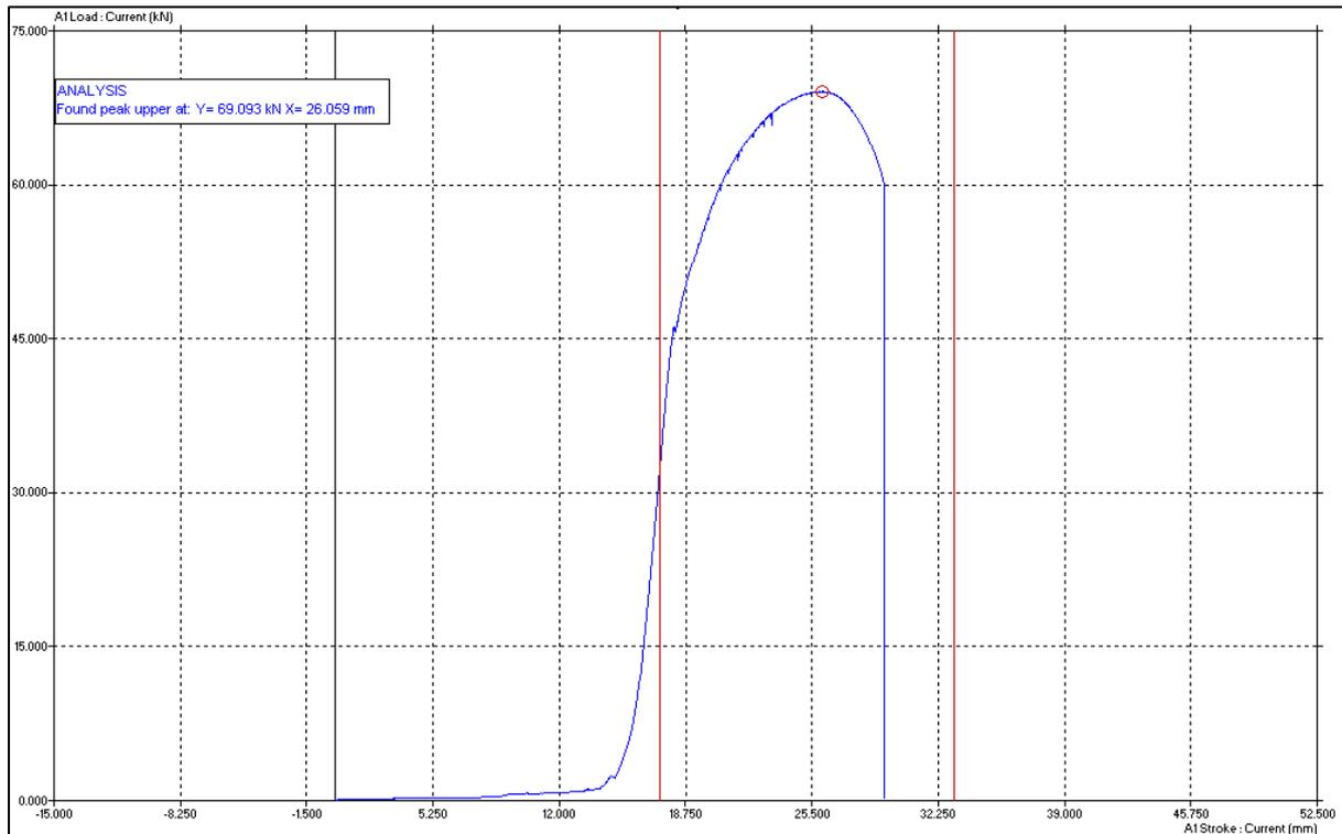
Figure 4.15: Force versus Strain for SA106B Steel (After Heat Treatment)
