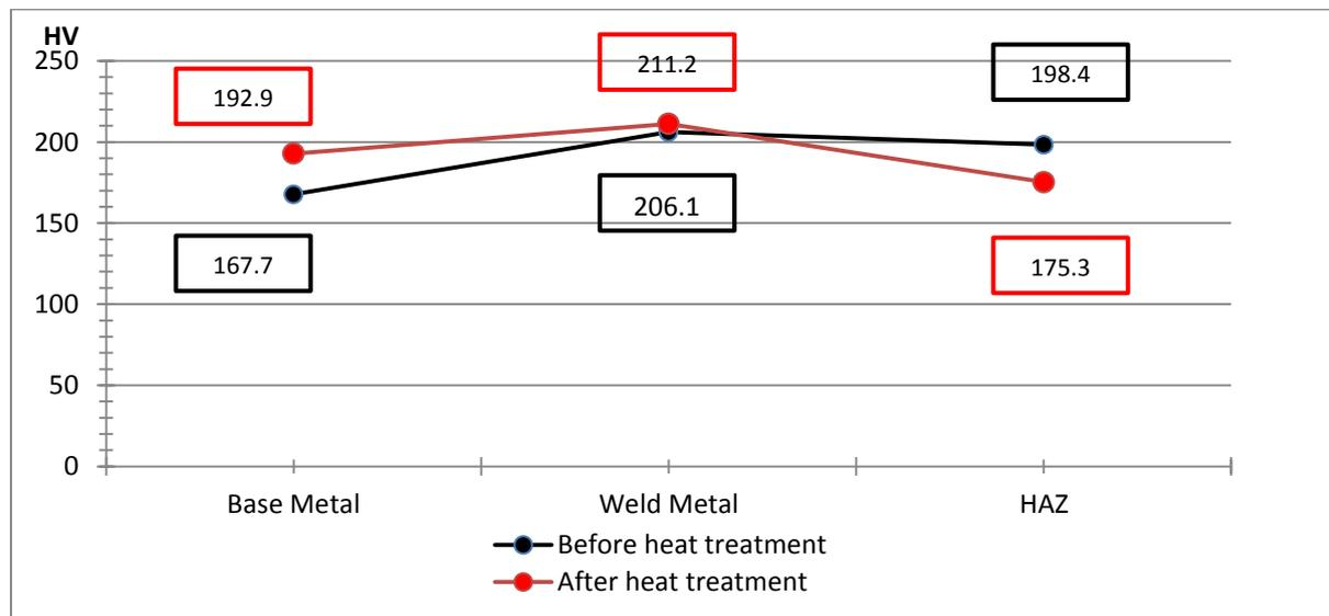
Figure 4.12: Mild steel hardness comparison before and after heat
