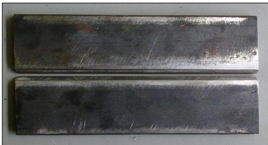
Figure 3.3: Bevel preparation
