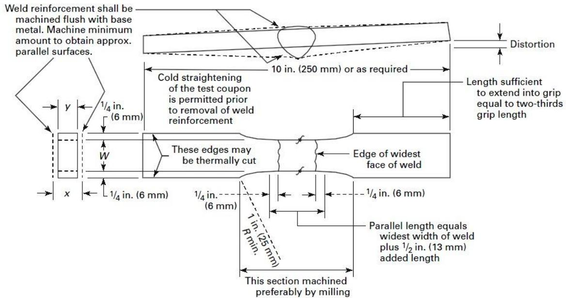
Figure 2.9: Tension specimen for plate (reference: ASME IX, 2007, QW-462)
