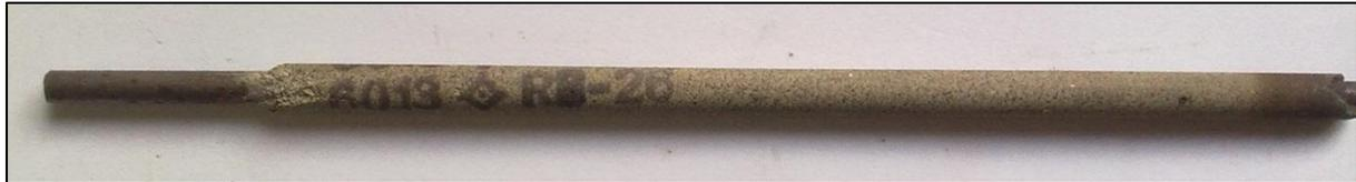
Figure 3.4: Electrode E6013 RB-26, 3mm diameter
