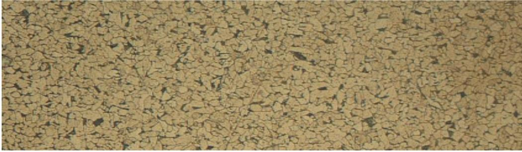
Figure 4.2: Base/Parent Metal microstructure under 100x magnification
