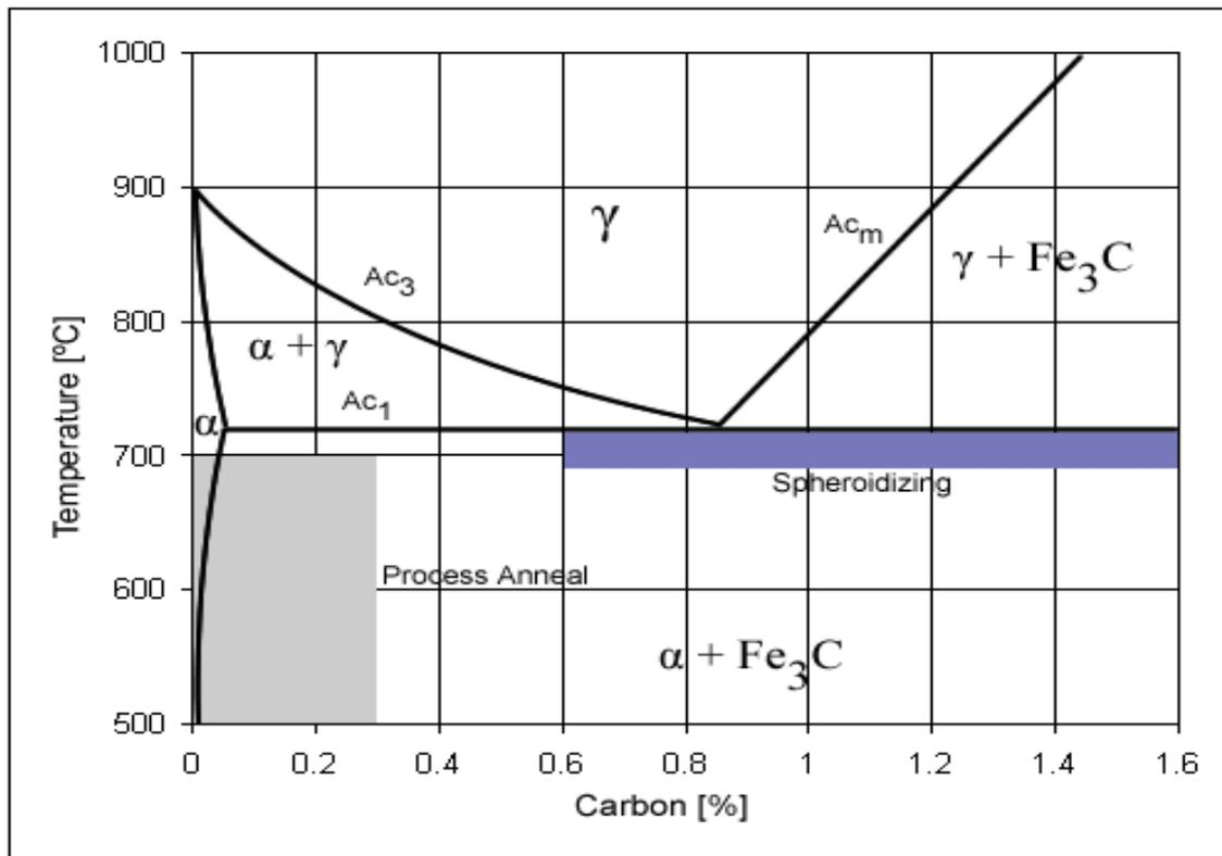
Figure 2.2: Heat Treatment Temperature on Phase Diagram
