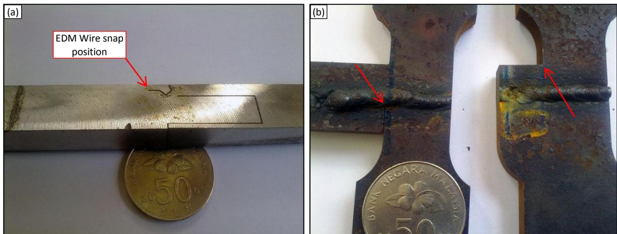
Figure 5.1: Example of sample unable to continue cutting.
