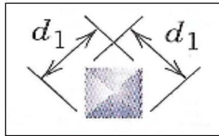
Figure 2.8: Example of Indentation Impression on test sample
