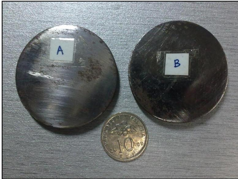
Figure 3.1: Test Sample for X-Ray Fluorescence
