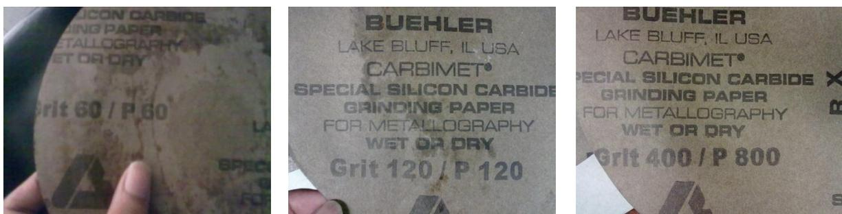
Figure 3.7: Example of sand papers discs
