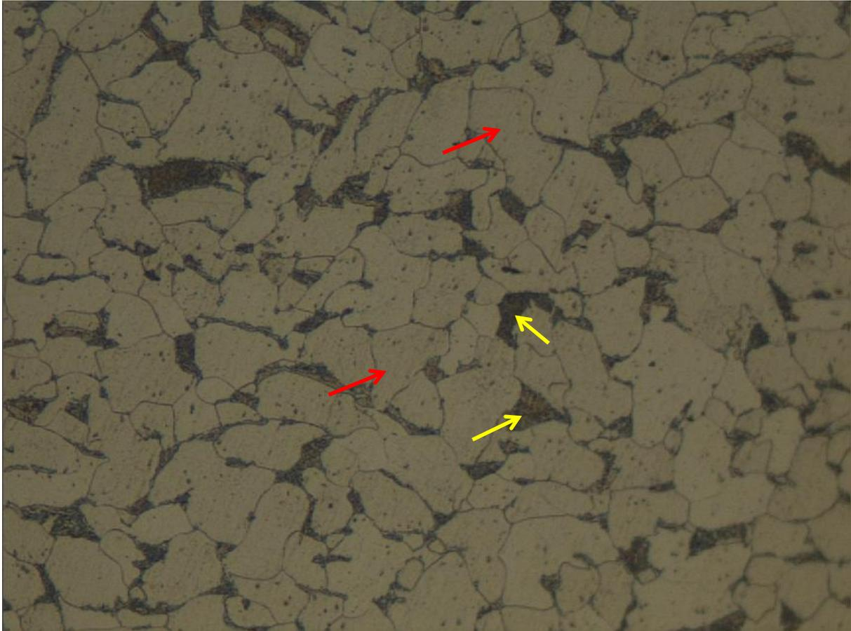
Figure 4.1: Mild Steel microstructure under 500x magnification by optical microscope.
