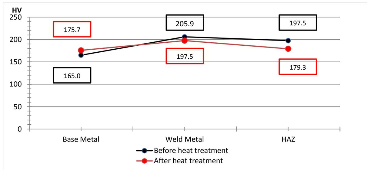
Figure 4.13: SA106B Steel hardness comparison before and after
