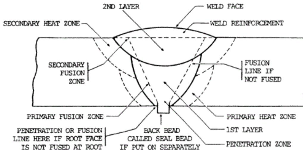
Figure 2.4: Terms of a Butt Welded Butt Joint
