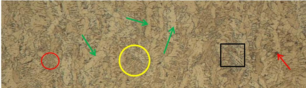
Figure 4.3: Weld/Filler Metal, also known as fusion zone microstructure under 100x magnification
