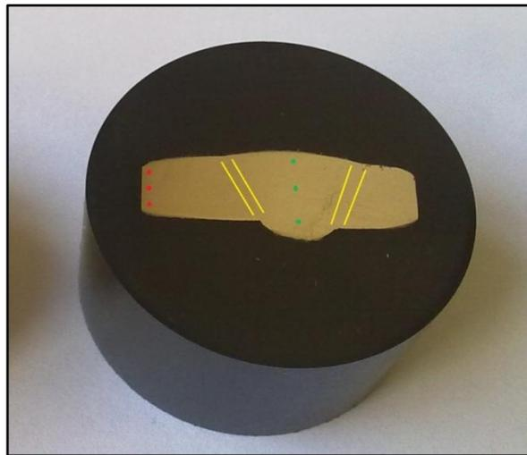
Figure 3.8: Hardness test area. (Red dot: base metal, green dot: weld metal, between yellow line: HAZ)
