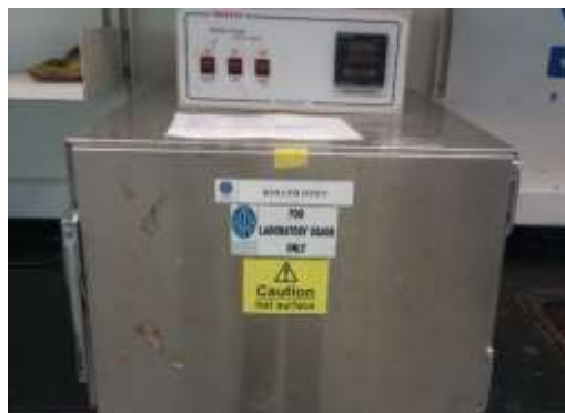
Figure 3.9: Fann Roller oven used
