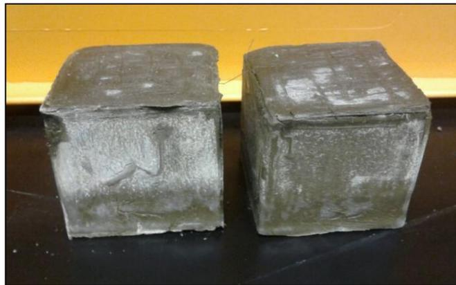
Figure 18. Cement samples that have been cured
