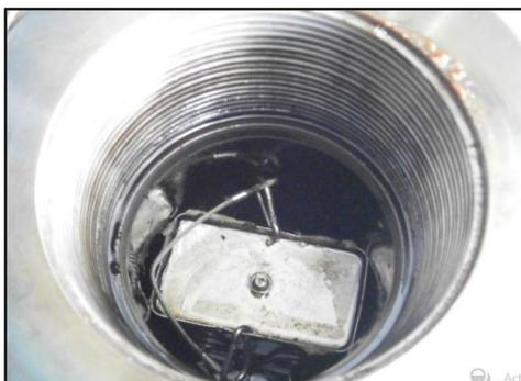
Figure 14. Molds are inserted into pressure vessel
