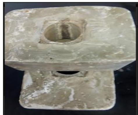
Figure 22. The remaininClass G Cement after coring process is done
