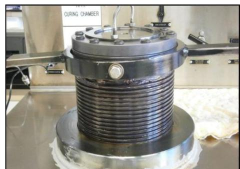
Figure 15. Cylinder plug is threaded into pressure vessel
