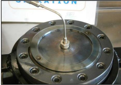
Figure 16. Thermocouple is inserted into pressure vessel
