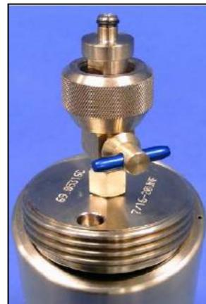
Figure 30. Top valve installed on grooved cap [58]
