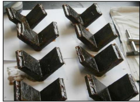
Figure 11. Greased curing molds
