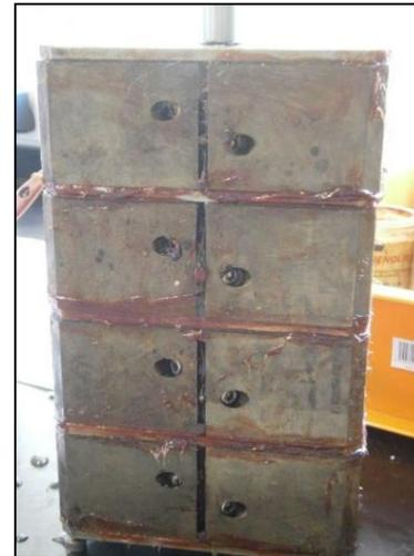
Figure 13. Curing molds are tied using thread
