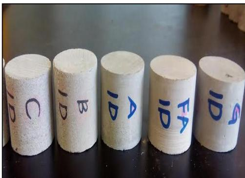
Figure 21. Cement sample after coring and trimming process
