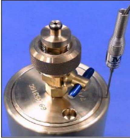
Figure 31. Thermocouple inserted through the hole on the cell [58]
