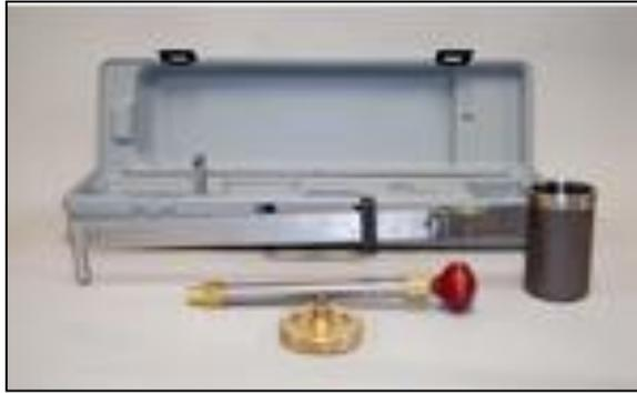
Figure 33. Pressurized mud density balance
