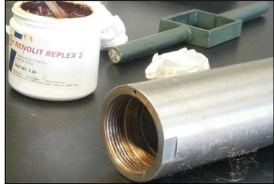
Figure 26. Greased cylinder cell
