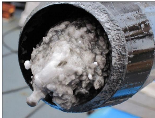
Figure 2.3: Gas hydrates formed in the pipeline.
