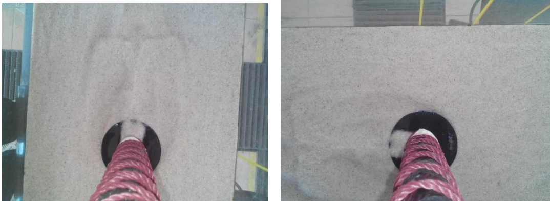
Scour Pattern: E3 ( b/D = 0.1 , \theta = 15^\circ with collar)
