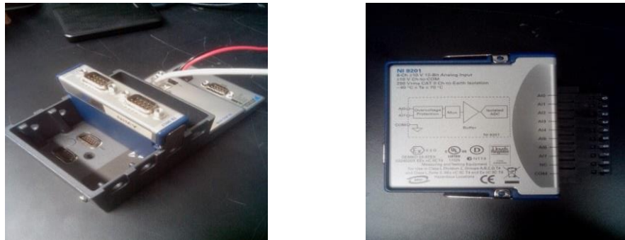
Fig.6: CompactRIO Real-Time Controller
