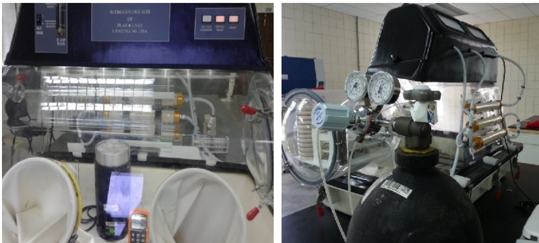
Fig. 12. Nitrogen box in CCR used to characterize humidity sensor
