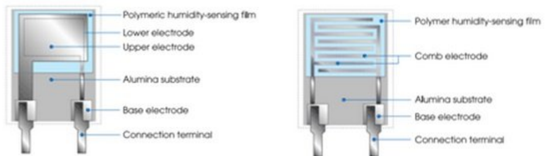
Fig. 2. Basic structure of capacitive and resistive humidity sensor[9]
