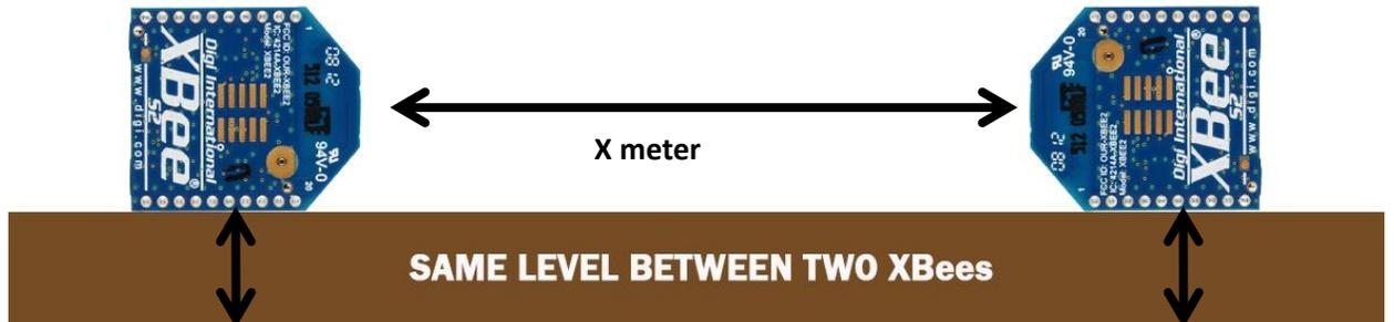
Figure 17: the XBees must be in the same level from the ground
