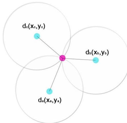
Figure 2: Intersection of three spheres in 2D using Trilateration [3]
