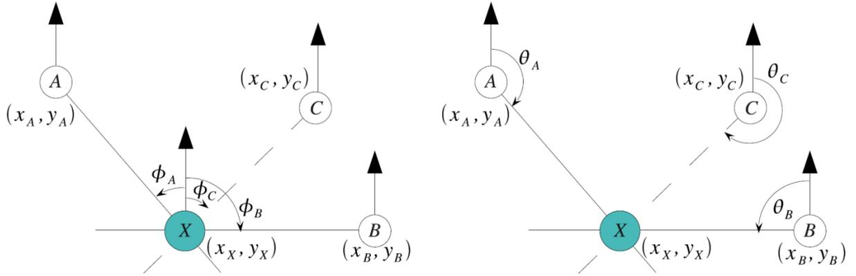
Figure 3: Angle of Arrival and Angle of Transmission [5]
