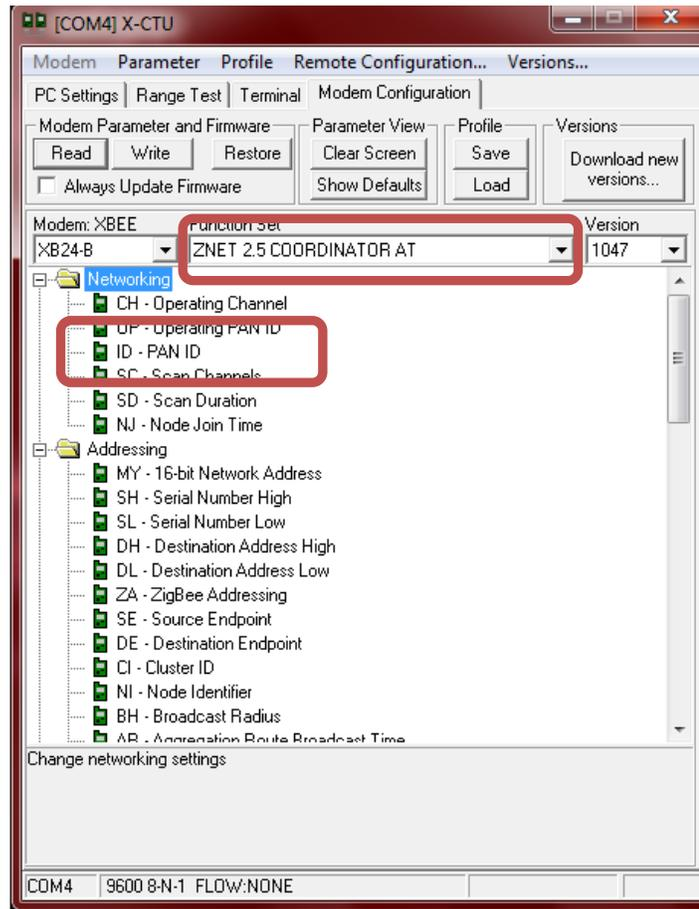
Figure 9: Coordinator AT firmware is loaded
