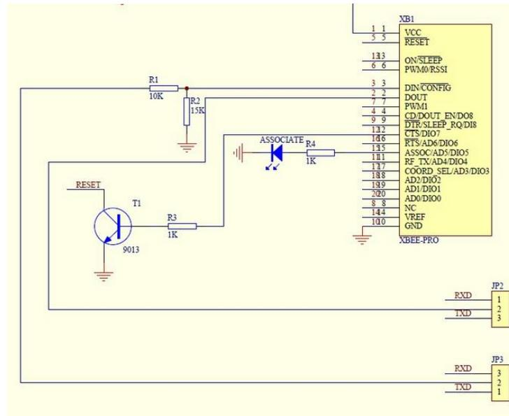
Figure 13: Schematic of XBee Shield
