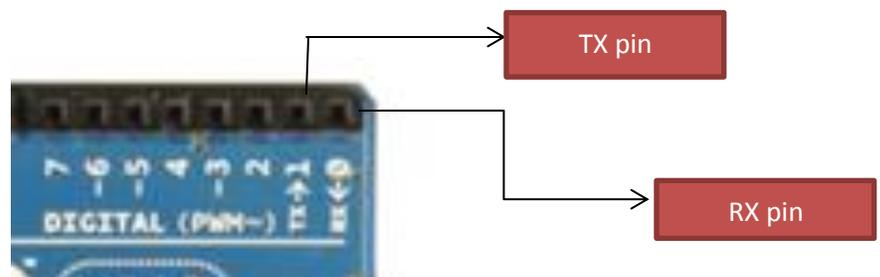
Figure 12: RX and TX pins on Arduino board
