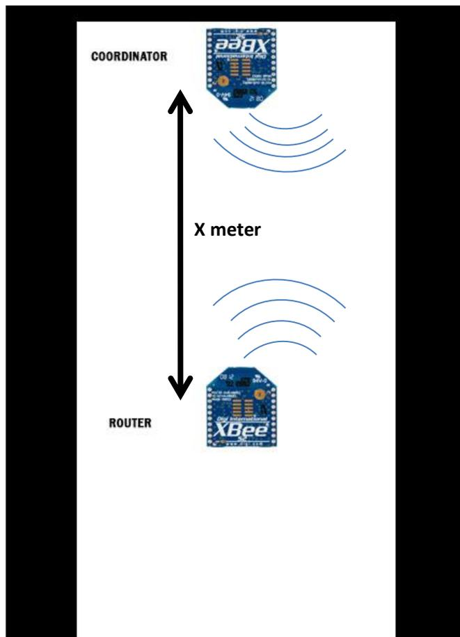
Figure 16: Range test Experiment Setup
