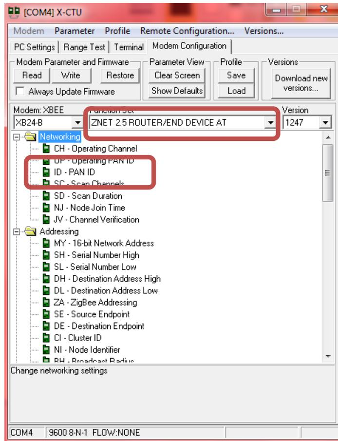
Figure 10: Router AT firmware is loaded
