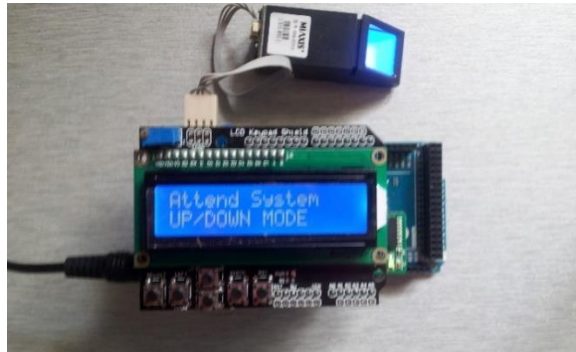
Figure 21: The Result of LCD Display Testing
