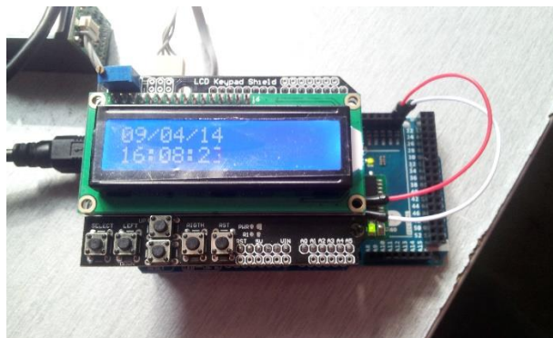
Figure 22: The Result of RTC Module Testing
