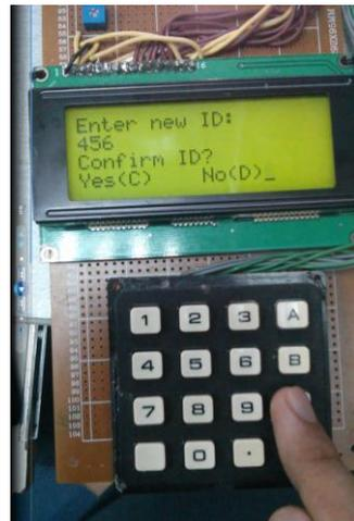
Figure 48: The tag is programmed with new ID, 456.
