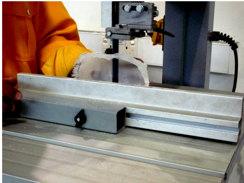
Figure 31: Electrical Saw Cutting Trough the Casing Base
