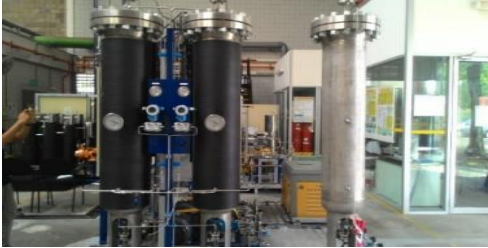
Appendix 1: Two pressure vessel and the open tank of the test rig
