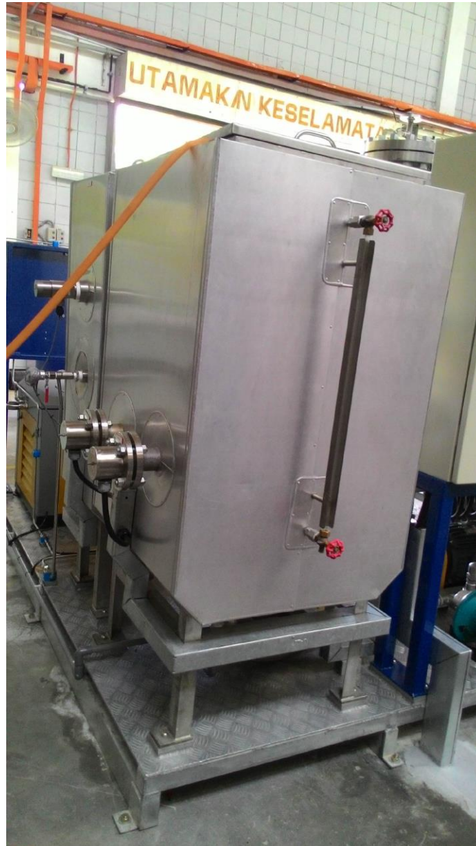
Appendix 3: Water tank with heater of the test rig
