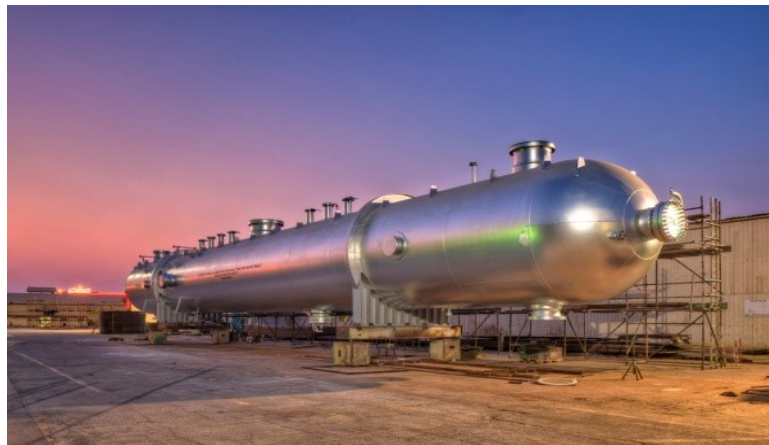
Figure 1: Typical Industrial Multiphase Separator (Source: (Craddock, 2014))
