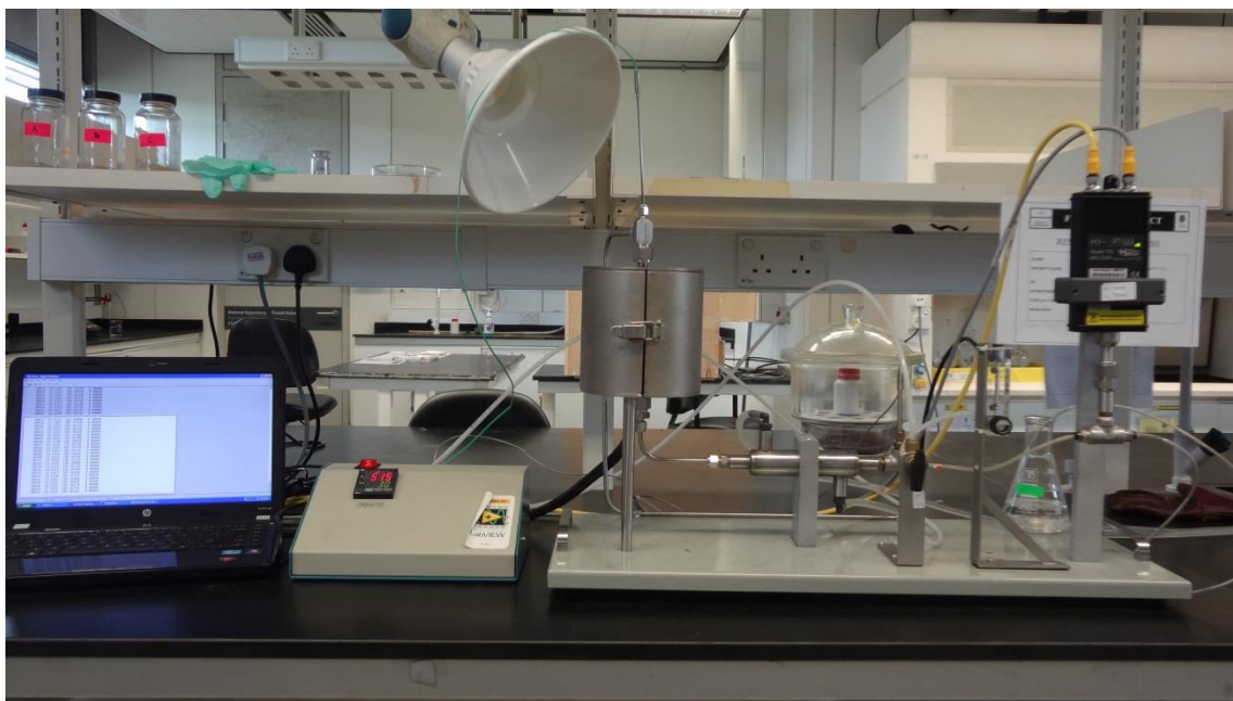
FIGURE 10: Experimental set-up for the methane decomposition
