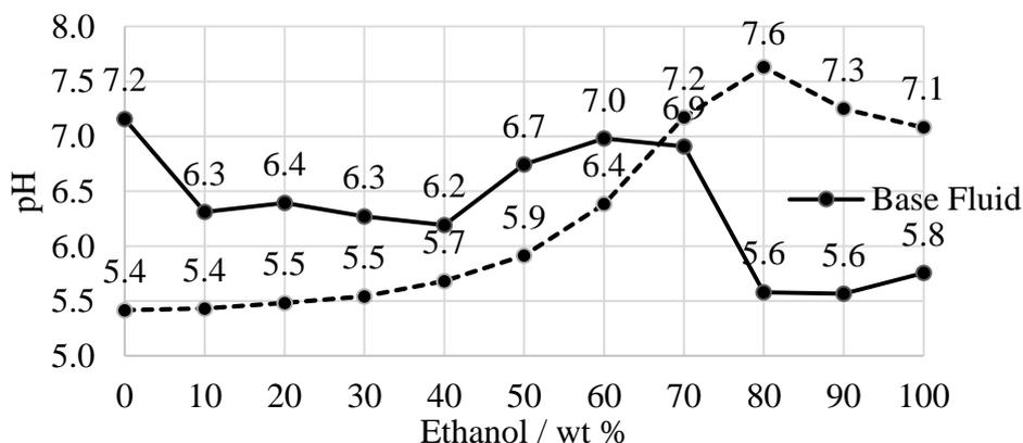
Figure 11: pH of base fluids and with alumina
