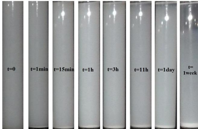
Figure 15: Sedimentation of alumina in 100% ethanol composition over time
