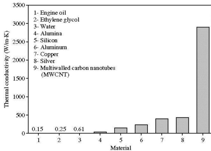
Figure 1: Thermal conductivity of typical materials at 300 K – Choi et al.
