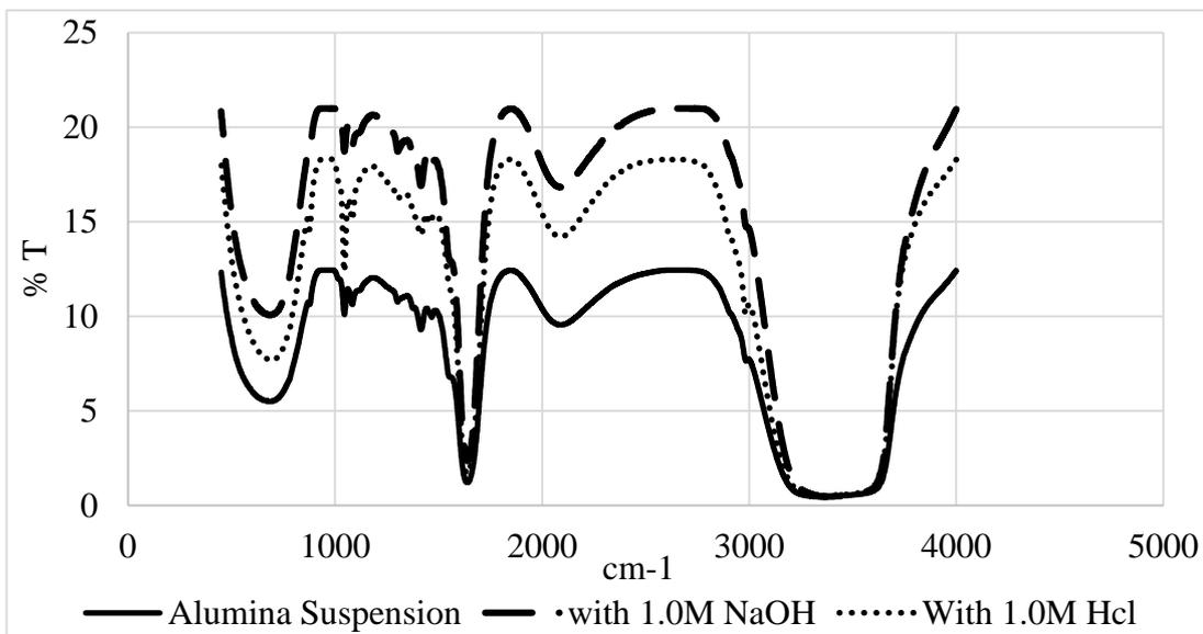
Figure 8: Spectra of alumina suspension and with 1.0M of Hcl and NaoH
