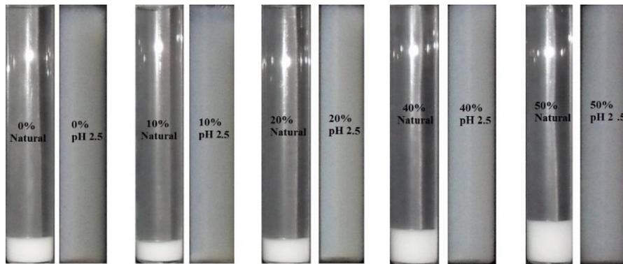
*Figure 17: Comparison between sedimentation of natural alumina suspension and at pH 2.5 after 11 hours*
