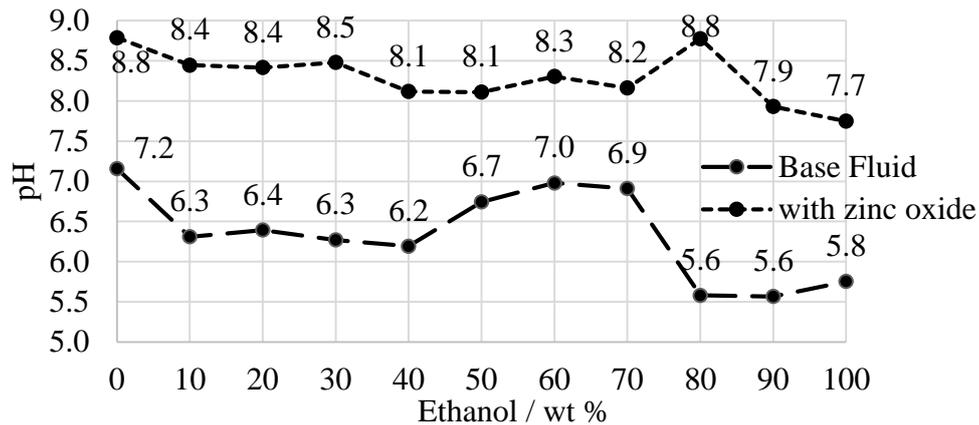
Figure 10: pH of natural base fluids and with zinc oxide
