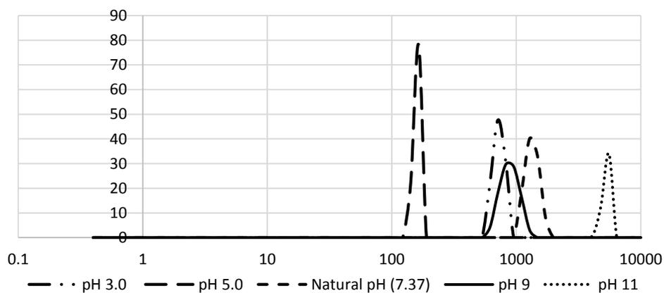
Figure 27: Particle size distribution for zinc oxide suspension at different pH values
