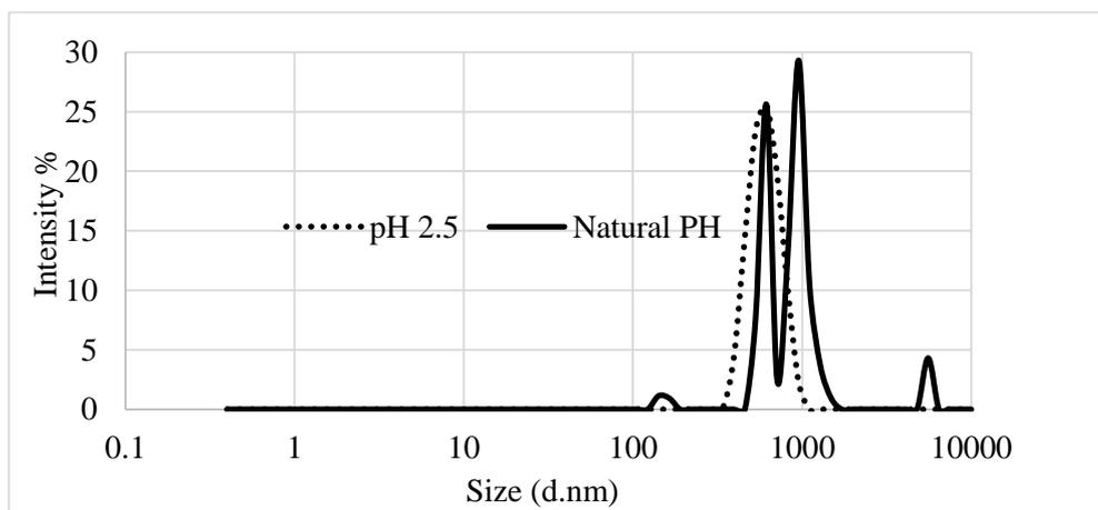
Figure 25: Particle size distribution for alumina suspension at pH 2.5 and natural pH
