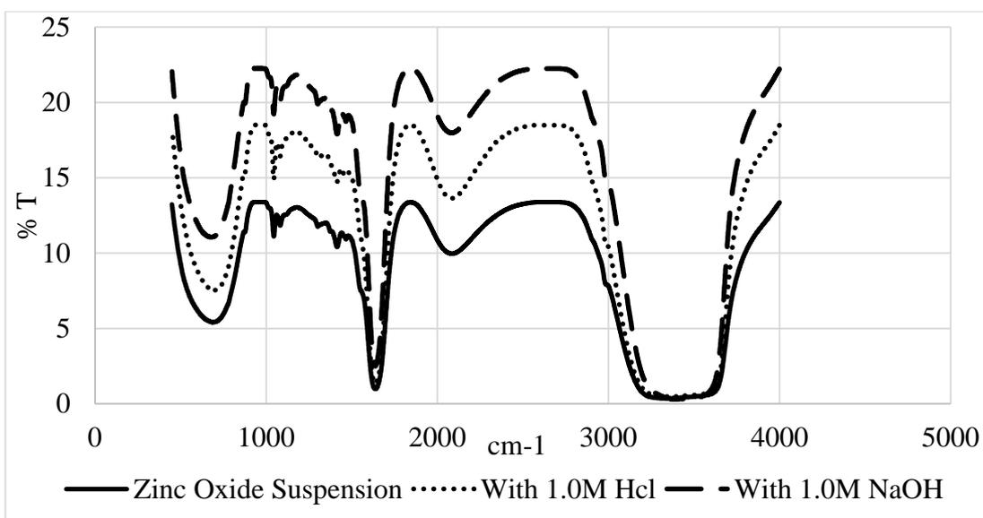
Figure 9: Spectra of zinc oxide suspension and with 1.0M of Hcl and NaOH
