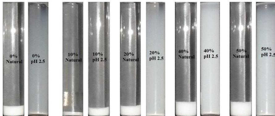
*Figure 18: Comparison between sedimentation of natural alumina suspension at pH 2.5 after 1 week*
