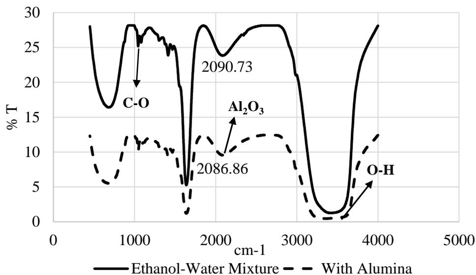
Figure 6: Spectra of ethanol-water mixture and alumina suspension
