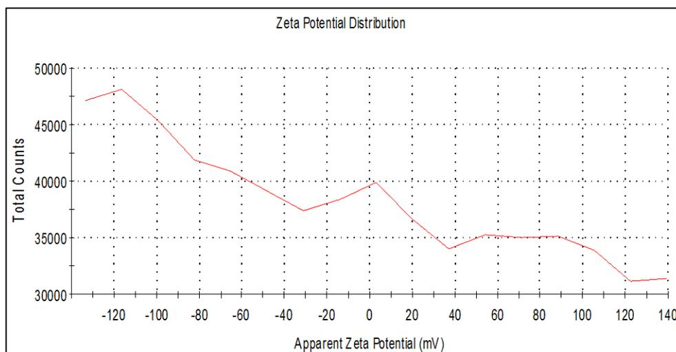
Figure 30: Zeta potential distribution of alumina suspension in 50% ethanol at pH 2.5
