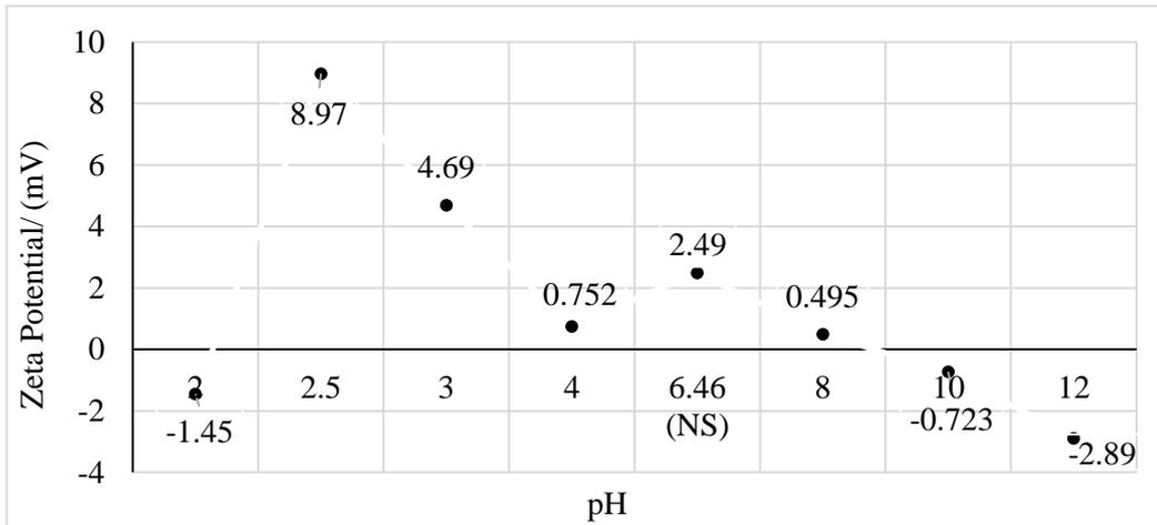
Figure 28: Zeta potential of alumina suspension in 50% ethanol concentration
