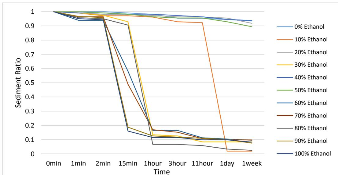
Figure 16: Graph of sediment ratio against time for alumina suspension at pH 2.5
