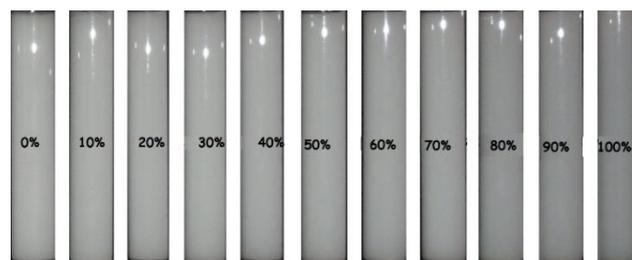
Figure 13: Sediment height for natural alumina suspension at  $t = 0$
