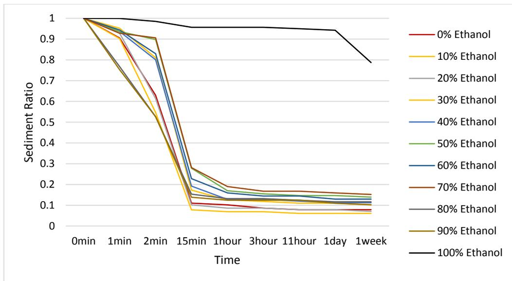
Figure 12: Graph of sediment ratio against time for natural alumina suspension
