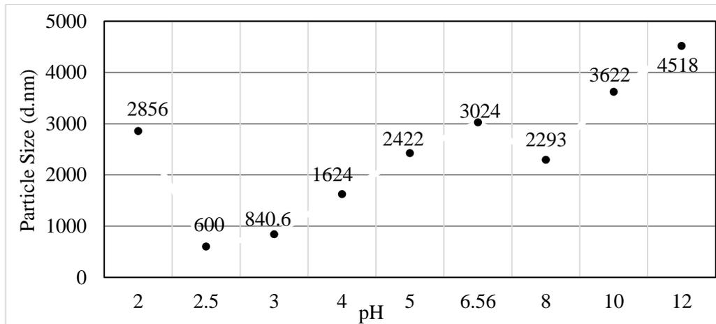
Figure 24: Size of alumina particles at different pH values
