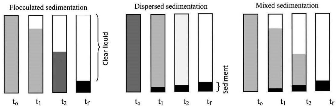
Figure 2: Three different types of settling behavior of suspensions with solid particles at different time intervals (Ilyas et al., 2013)
