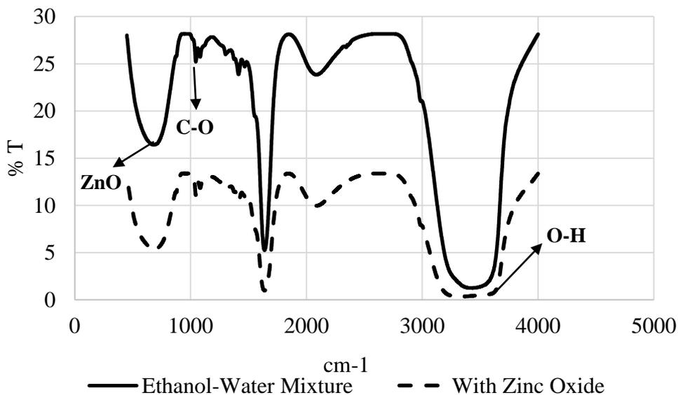
Figure 7: Spectra of ethanol-water mixture and zinc oxide suspension
