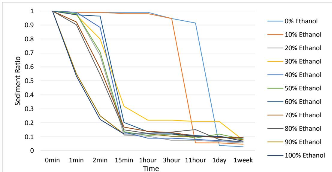
Figure 20 Graph of sediment ratio against time for alumina suspension at pH 4.0
