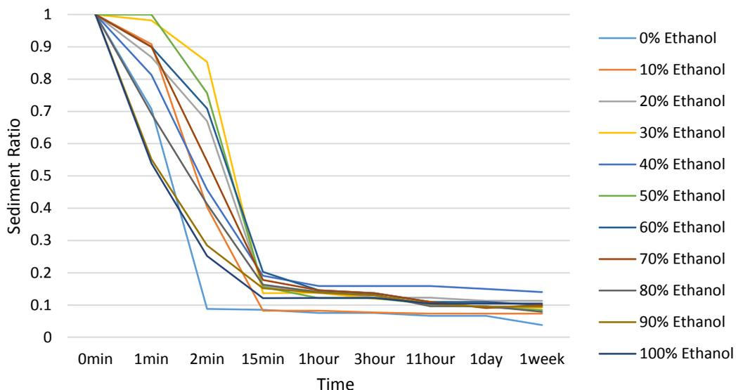
Figure 21 Graph of sediment ratio against time for alumina suspension at pH 8.5
