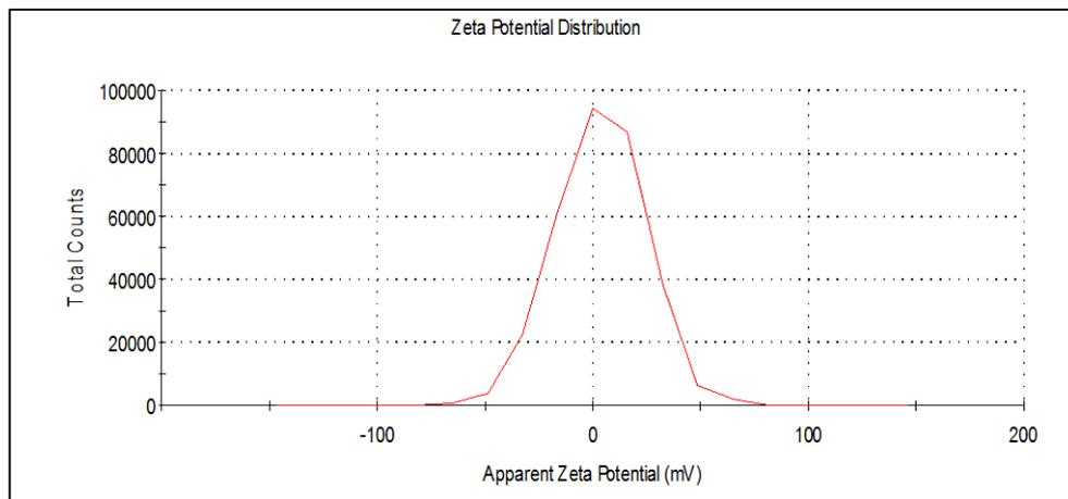
Figure 29: Zeta potential distribution of alumina suspension in 50% ethanol at natural pH
