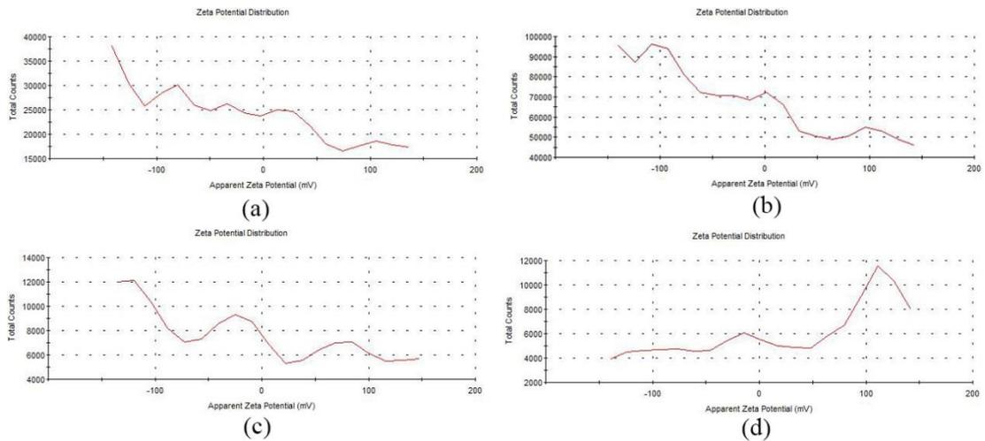
Figure 32: Zeta potential distribution of zinc oxide suspension in 50% ethanol at (a) natural pH (b) pH 3.0 (c) pH 5 (d) pH 9
