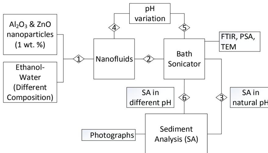
Figure 4: Flow diagram of the experimental procedure
