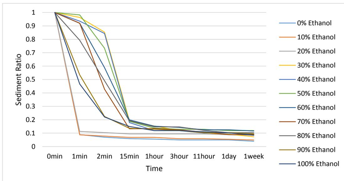
Figure 22 Graph of sediment ratio against time for alumina suspension at pH 10.5
