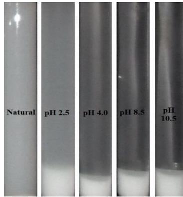
Figure 19: Comparison between the alumina suspensions in 100% ethanol at different pH after 15 minutes
