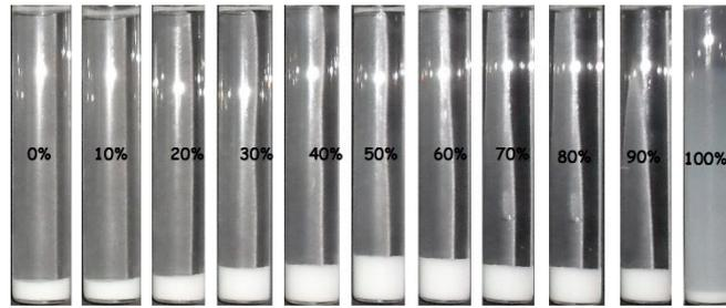
Figure 14: Sediment Height for natural alumina suspension at  $t = 1$  Week
