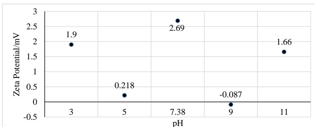
Figure 31: Zeta potential of zinc oxide suspension in 50% ethanol concentration
