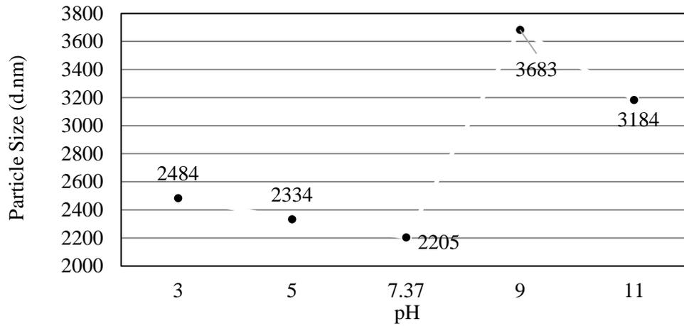
Figure 26: Particle size for zinc oxide suspension at different pH
