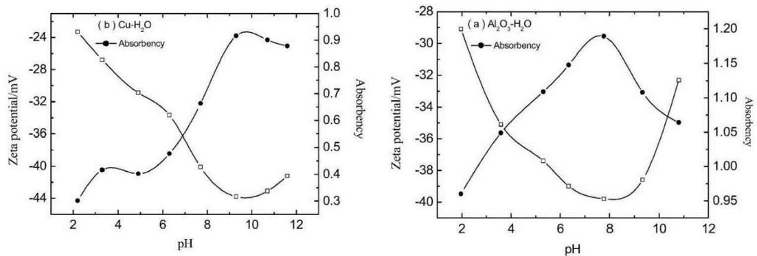
Figure 3: Effect of pH on zeta potential of nano-suspensions with SDBS dispersants.
