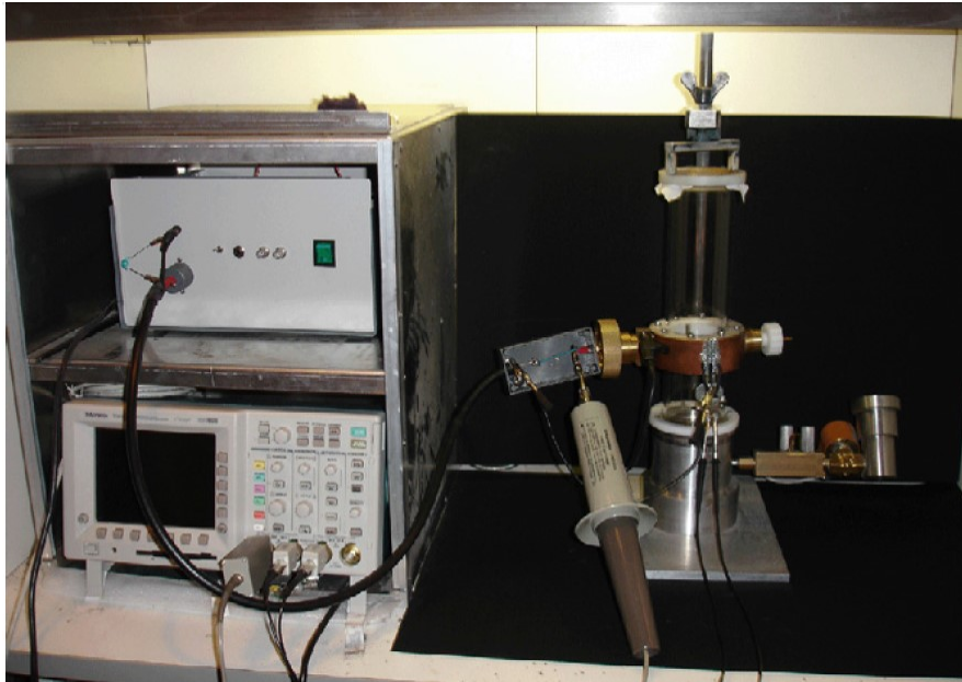
Figure 7: The spark generator, the spark energy measurement system and dust explosion chamber.
