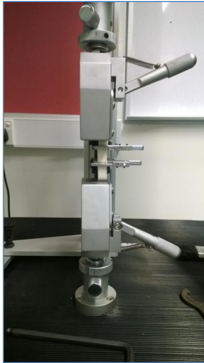
Figure 13: Placement of foam strip with the tensile strength machine
