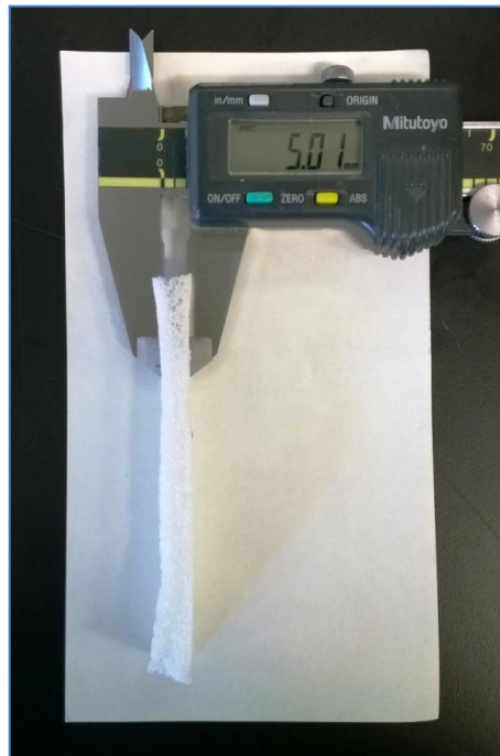
Appendix 2: Determination of strip thickness using a vernier calliper
