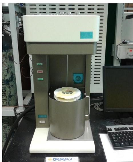
The COP-1 sample undergoes pre-treatment at 150°C under vacuum for 2 hours as seen in Figure 6 before adsorption test is carried out.
