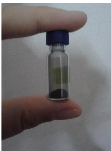
Figure A 9 Deactivation of catalyst due to carbon formation
