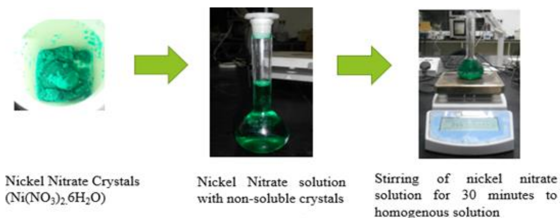
Figure 6 Steps for the preparation of 0.1 g/mL of Ni standard solution
