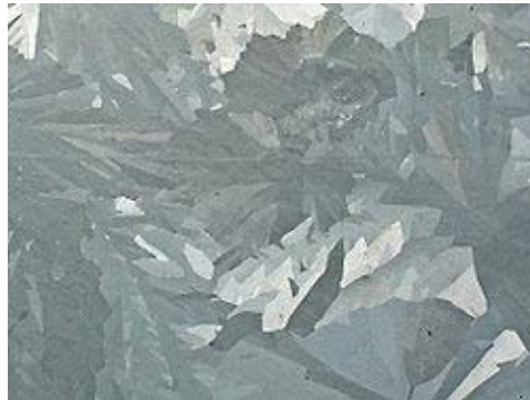
Figure 2: Crystalline surface of a hot-dip galvanized surface
