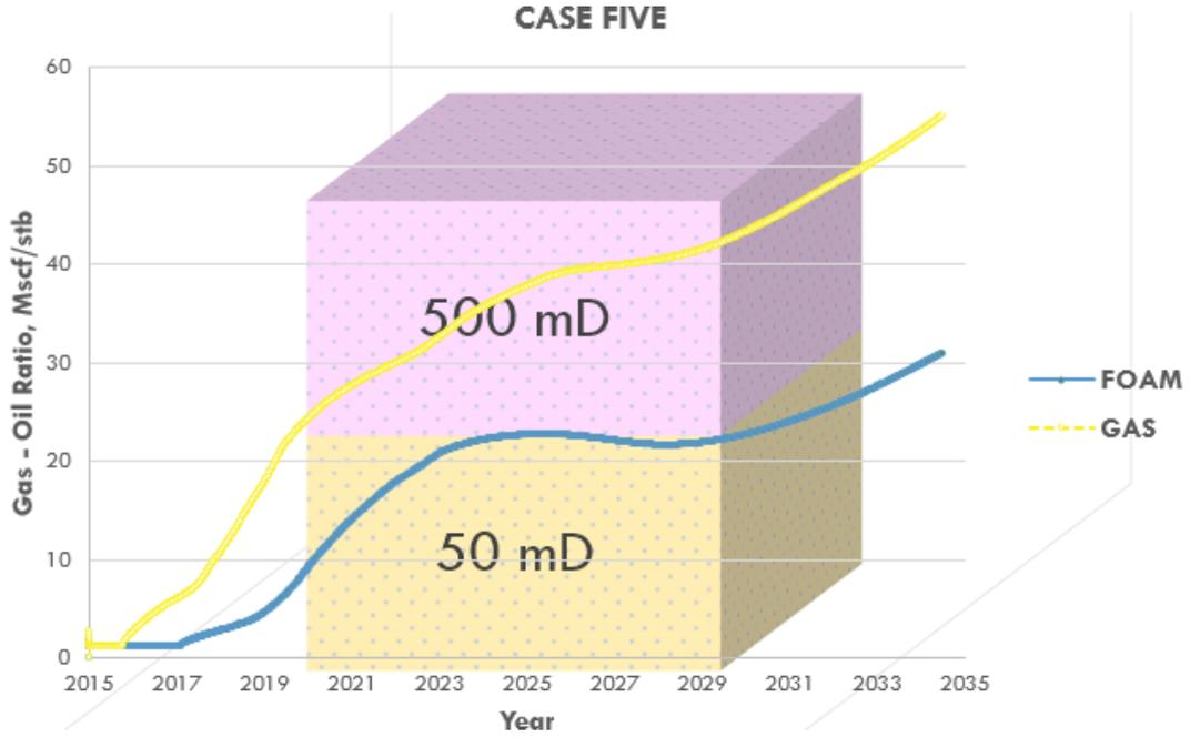
Figure 4.11: Gas - Oil Ratio: Case Five (High – permeability on Top)
