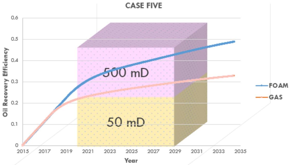
Figure 4.22: Oil Recovery Efficiency: Case Five (High – permeability on Top)
