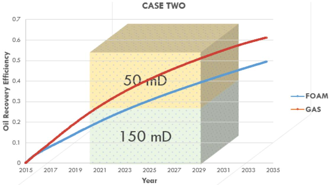
Figure 4.14: Oil Recovery Efficiency: Case Two (Low – permeability on Top)
