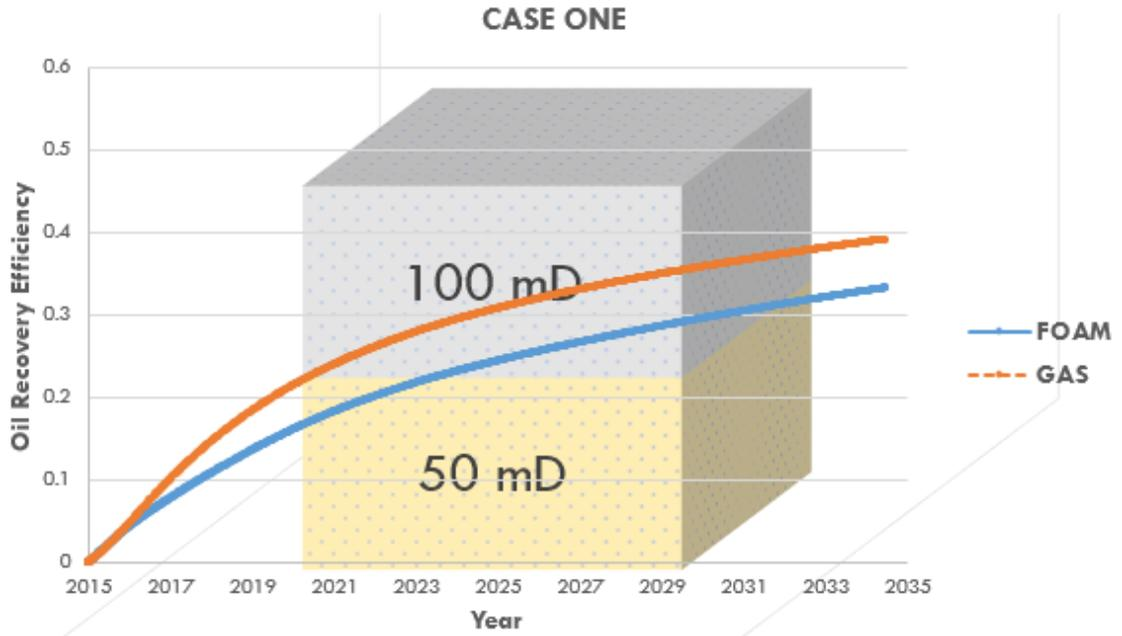
Figure 4.18: Oil Recovery Efficiency: Case One (High – permeability on Top)
