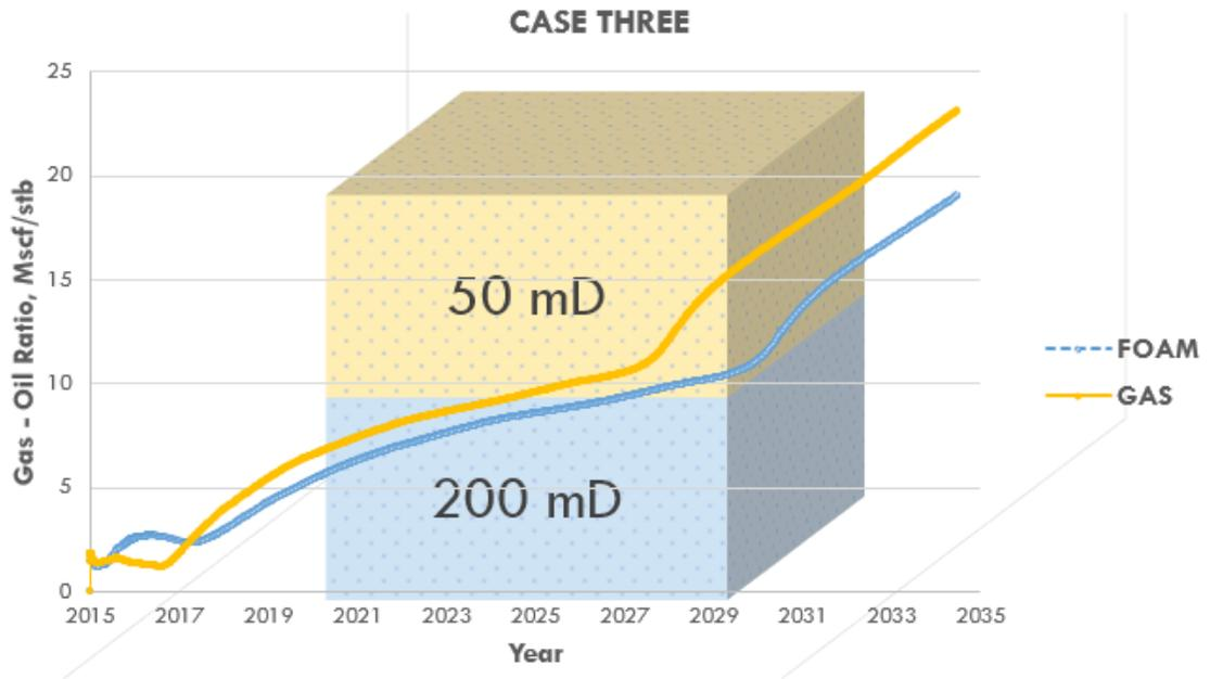
Figure 4.3: Gas - Oil Ratio: Case Three (Low – permeability on Top)
