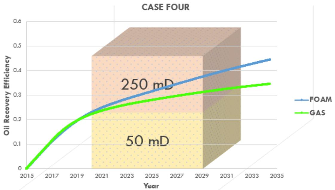
Figure 4.21: Oil Recovery Efficiency: Case Four (High – permeability on Top)
