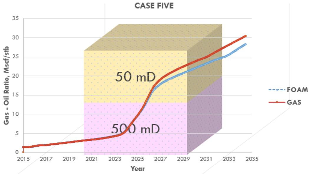
Figure 4.5: Gas - Oil Ratio: Case Five (Low – permeability on Top)
