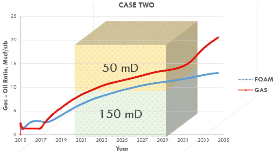
Figure 4.2: Gas - Oil Ratio: Case Two (Low – permeability on Top)
