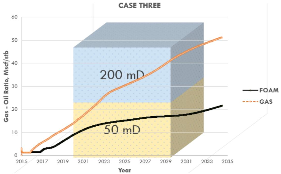
Figure 4.9: Gas - Oil Ratio: Case Three (High - permeability on Top)
