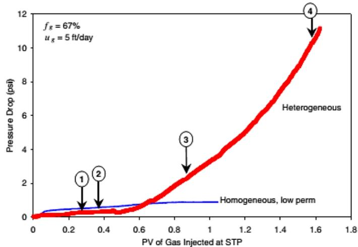
Figure 2.6: Pressure Drop during Foam Flooding Experiments. (Tanzil *et al.*, 2002)
