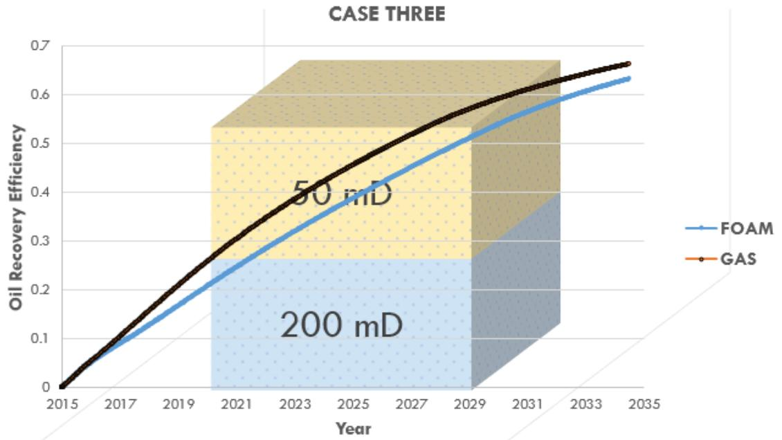
Figure 4.15: Oil Recovery Efficiency: Case Three (Low – permeability on Top)
