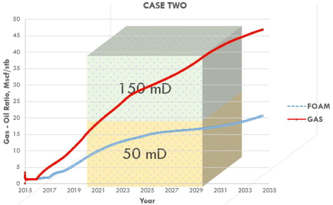
Figure 4.8: Gas - Oil Ratio: Case Two (High – permeability on Top)
