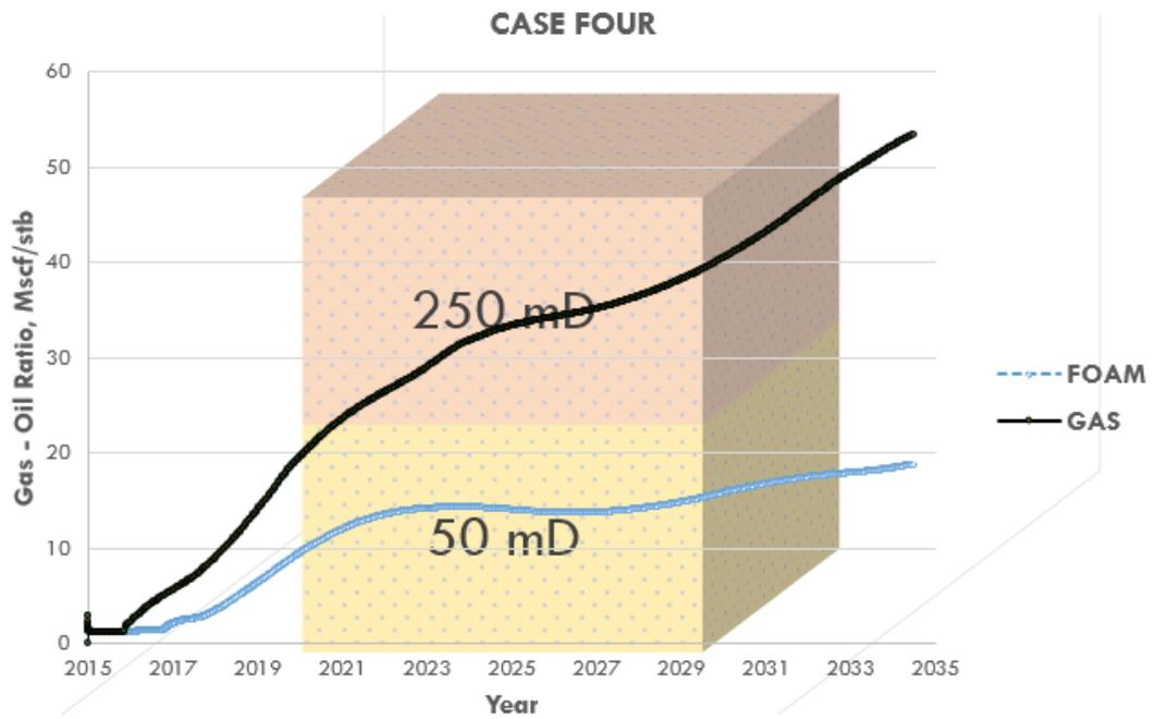
Figure 4.10: Gas - Oil Ratio: Case Four (High - permeability on Top)
