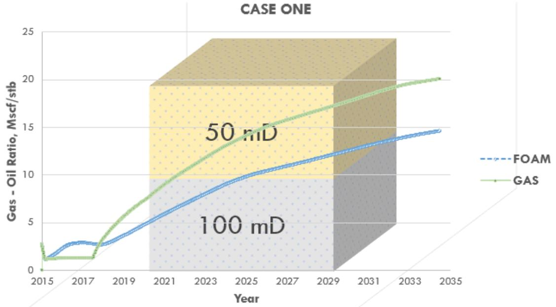
Figure 4.1: Gas - Oil Ratio: Case One (Low – permeability on Top)
