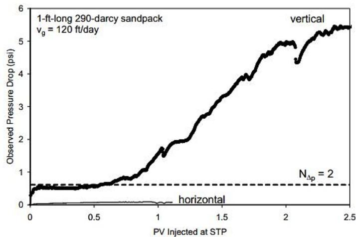
Figure 2.7: Pressure Drop in Horizontal and Vertical Sand-packs (Tanzil *et al.*, 2002)
