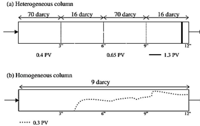
Figure 2.5: Foam Flood Fronts in (a) Horizontal Heterogeneous, (b) Horizontal Homogeneous Sand-packs (Tanzil et al., 2002)
