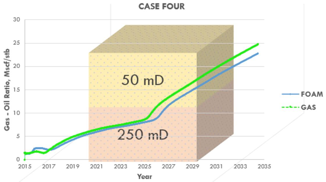
Figure 4.4: Gas - Oil Ratio: Case Four (Low – permeability on Top)
