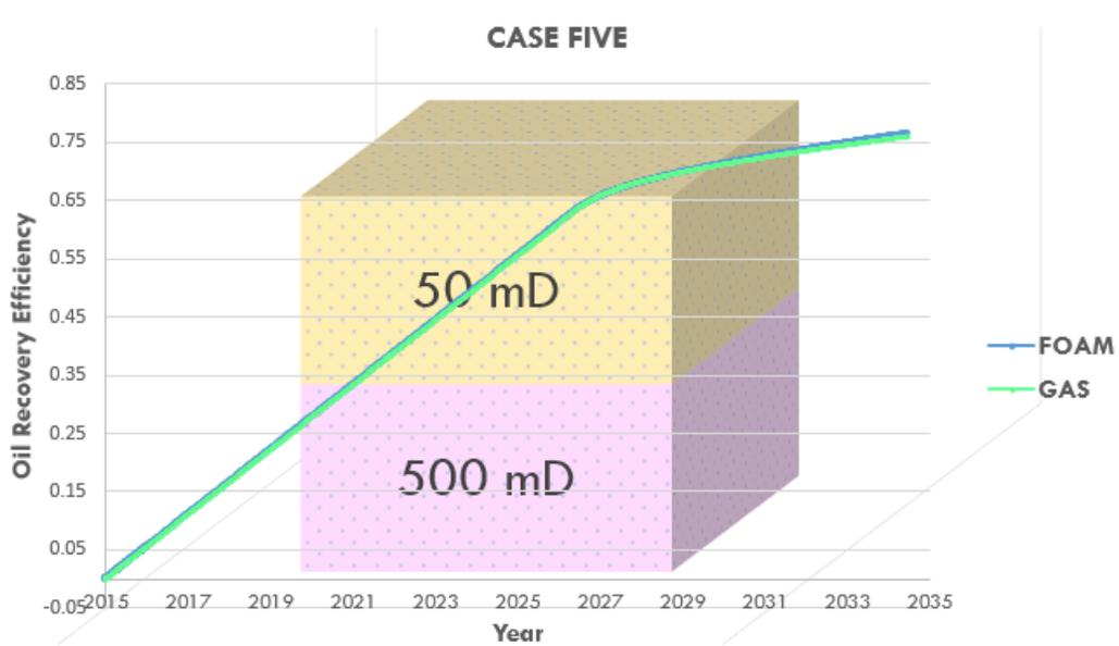
Figure 4.17: Oil Recovery Efficiency: Case Five (Low – permeability on Top)
