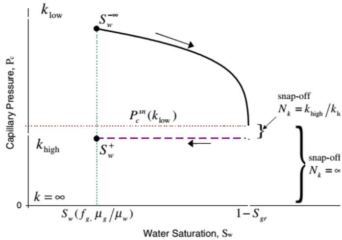
Figure 2.3: Snap-off Mechanism at Sudden Permeability Increase (Tanzil *et al.*, 2002)
