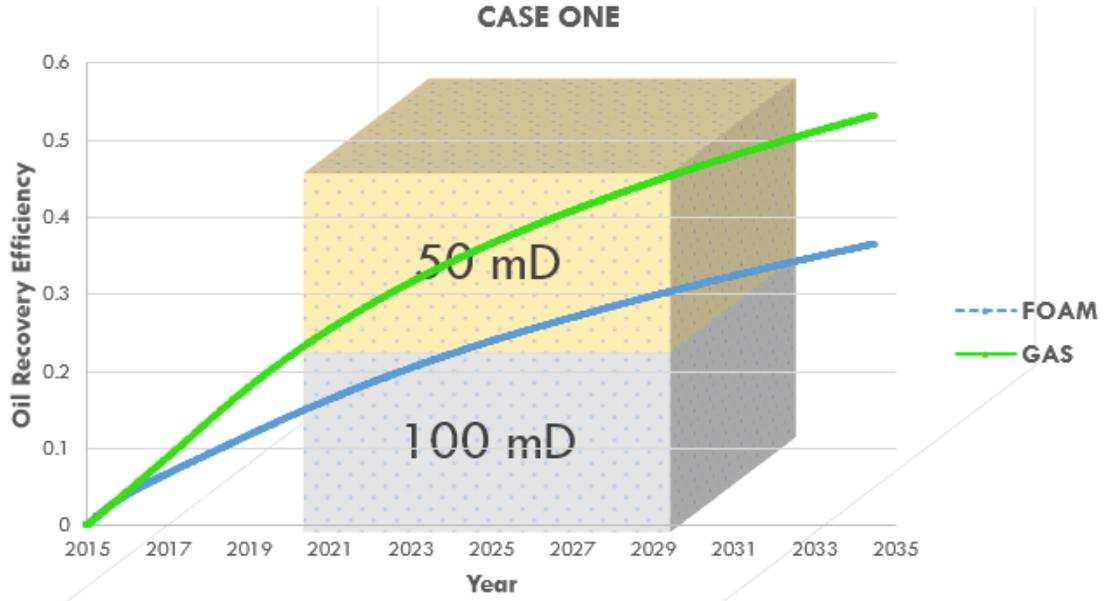
Figure 4.13: Oil Recovery Efficiency: Case One (Low – permeability on Top)
