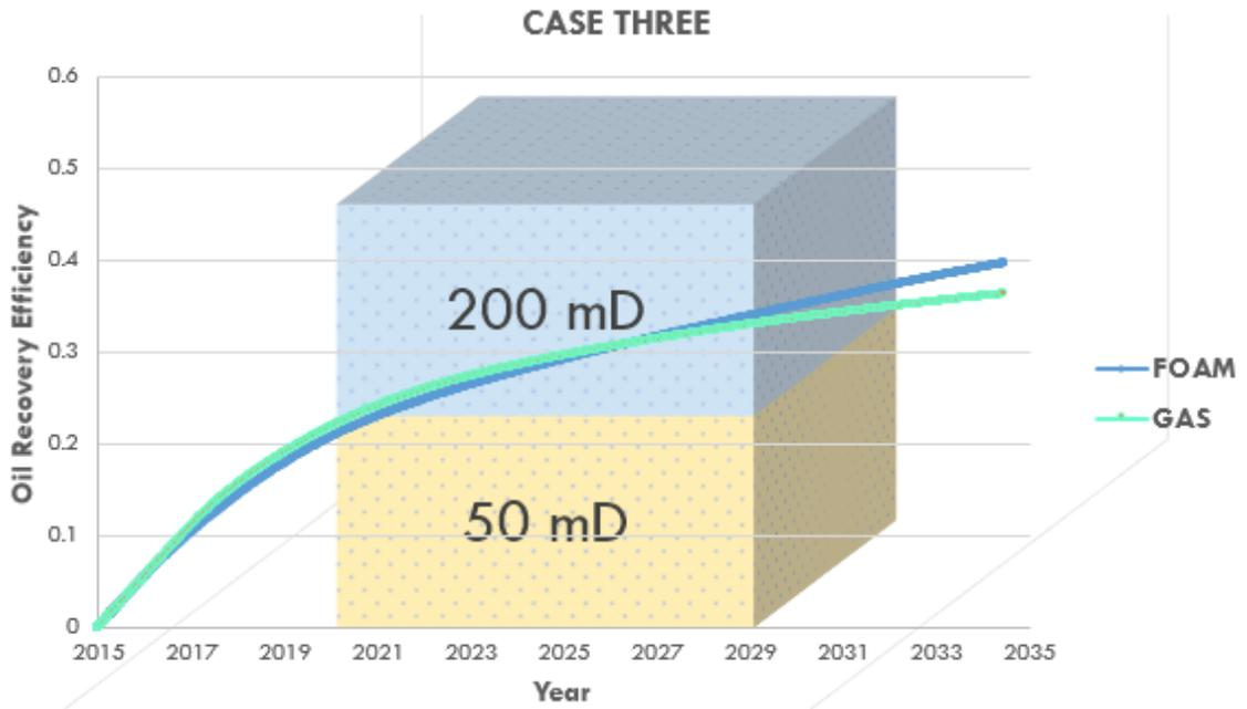
Figure 4.20: Oil Recovery Efficiency: Case Three (High – permeability on Top)
