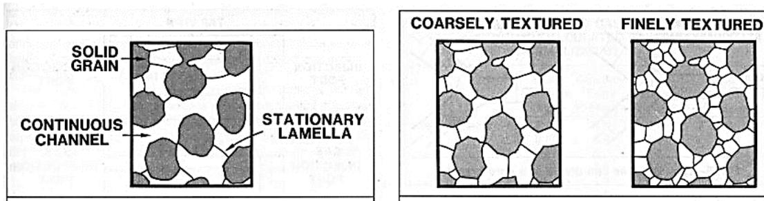
Figure 2.1: Continuous Foam (left) and Discontinuous Foam (right) (Falls *et al.*, 1988)
