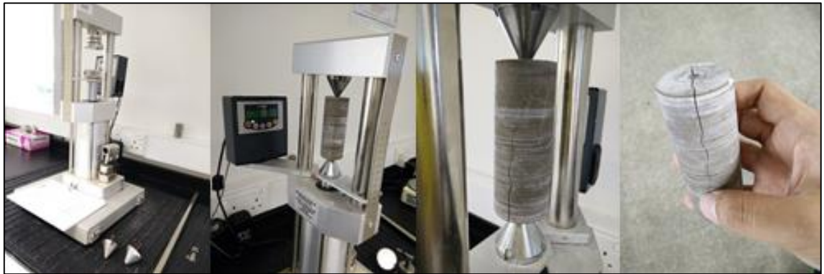
FIGURE 3.12: The point load test machine to calculate the uniaxial compressive strength and a sample tested.
