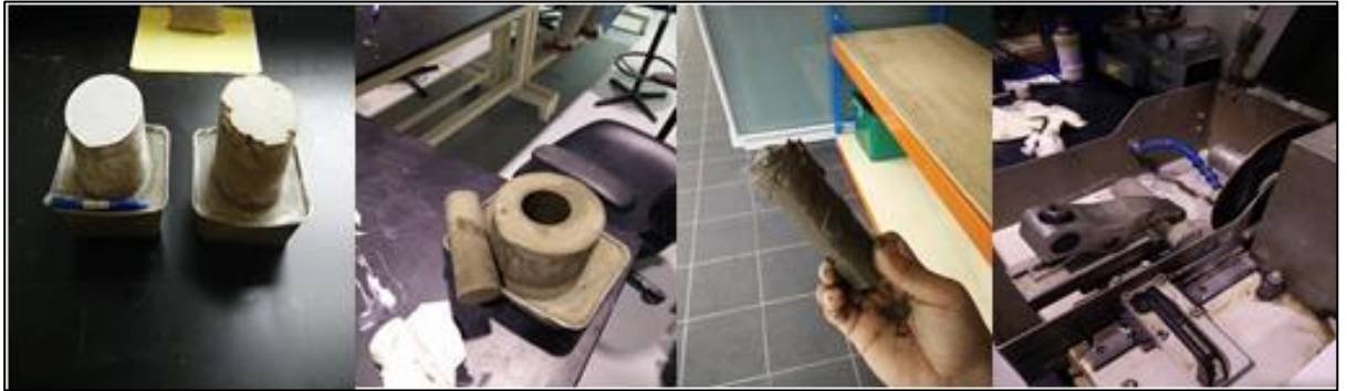
FIGURE 3.9: The coring process to produce cylindrical- shaped geopolymer cement
