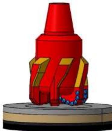
Figure 18 3D Model of PDC bit in assembly design
