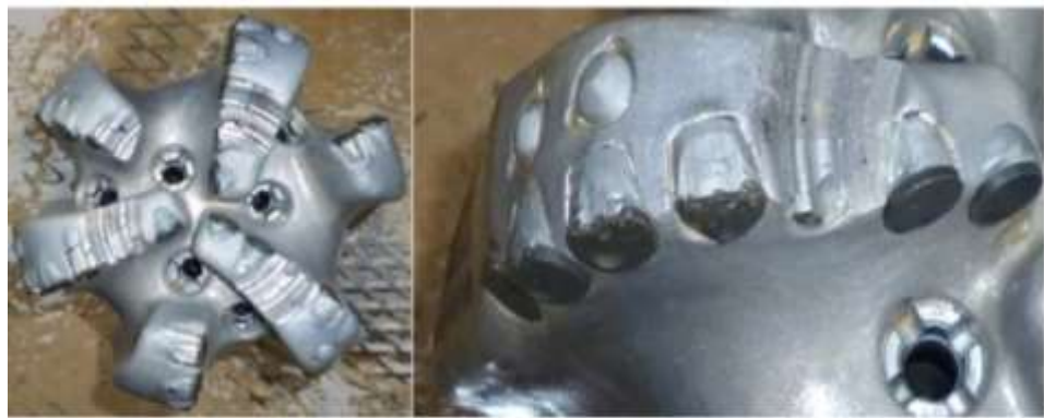
Figure 7 Bit condition after drilled in multi-layer formation. Source from Kamatov (2013), Hybrid Drill Bit For Horizontal Drilling In Highly Interbedded Formations Of Timano-Pechora Arctic Fields
