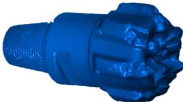
Figure 14 3D CAD Model of PDC Drill Bit
