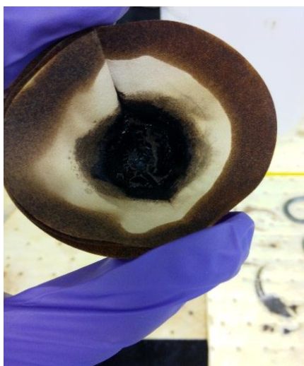
Figure 16: Asphaltene and coke precipitation after 60 minutes subcritical water treatment
