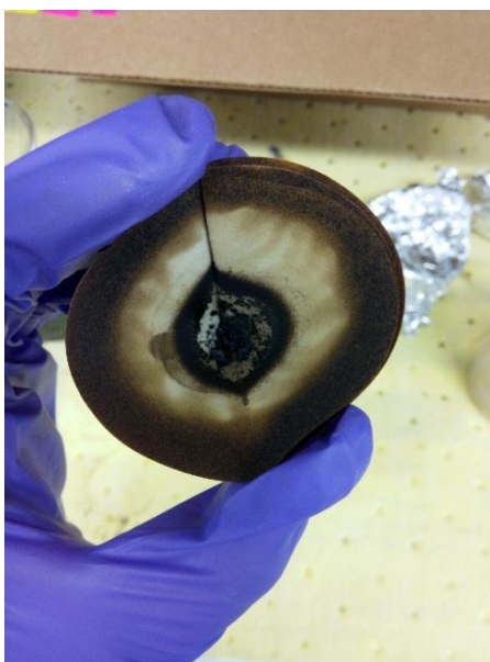
Figure 17: Asphaltene and coke after subcritical water treatment for 90 minutes
