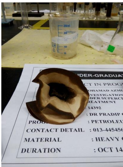
Figure 14: Asphaltene and Coke Precipitation
