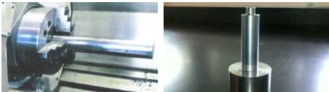
Figure 5: (a) Set up tool steel for fabrication of FSW welding tool. (b) Cylindrical pin tool after fabricated using CNC Lathe Turning Machine
