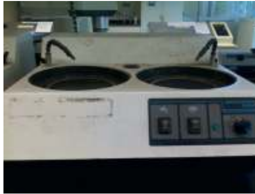
Figure 11: MetaServ 2000 Grinder Machine
