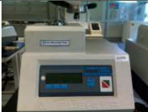
Figure 10: Auto Mounting Press Machine
