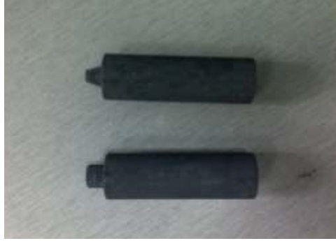
Figure 8: FSW tools after undergo heat treatment process
