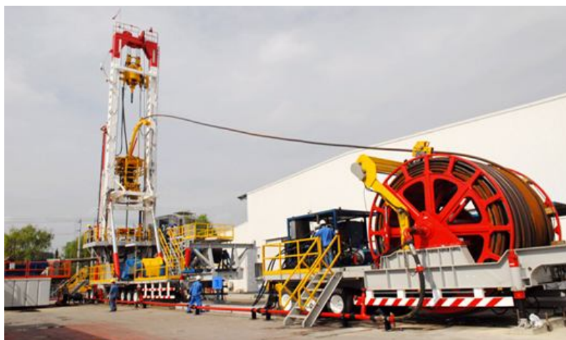
Figure 1: Portable Coiled Tubing Drilling Unit
